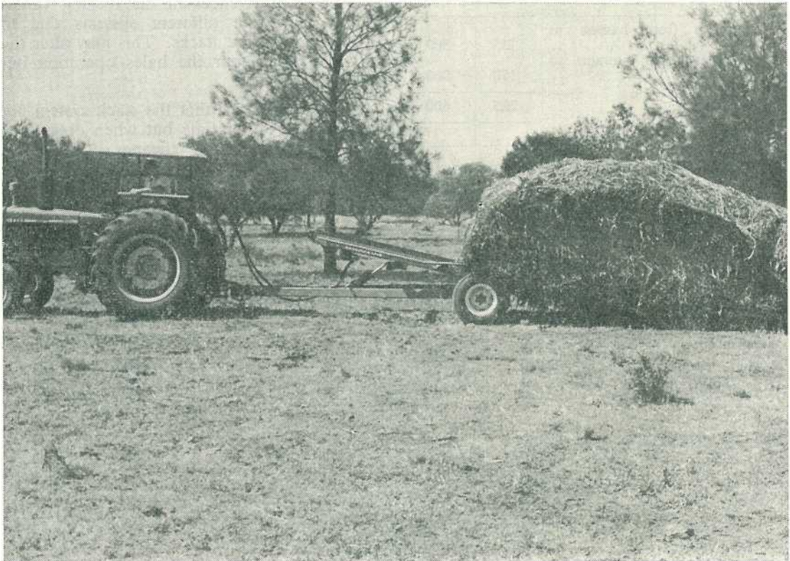
Stacks are easily loaded and unloaded with the stackmover trailer.
