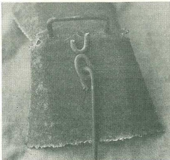
Plate 8. Mike starts the bends at the top of the bell first and then he starts the bends for the sides. He uses a light hammer to start these bends. Next, Mike brazes the keeper and tongue into position. The tongue swivels on two chain links, one of which is cut.
