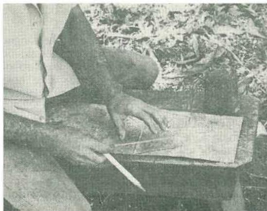
Plate 3. A template for the bells can be made by measuring any horse bell. Remember, the sides of the bell overlap.
