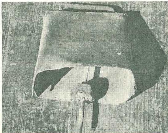
Plate 10. A heavy nut makes a good hammer. The hammer is in the correct position when its bottom edge is 2 to 3 mm below the bottom edge of the bell.
