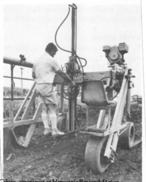
Gerry Gibson, agronomist at Hermitage Research Station, operating the Department's 'moon buggy', a mobile soil sampler especially suited to plot and farmer crop trials
