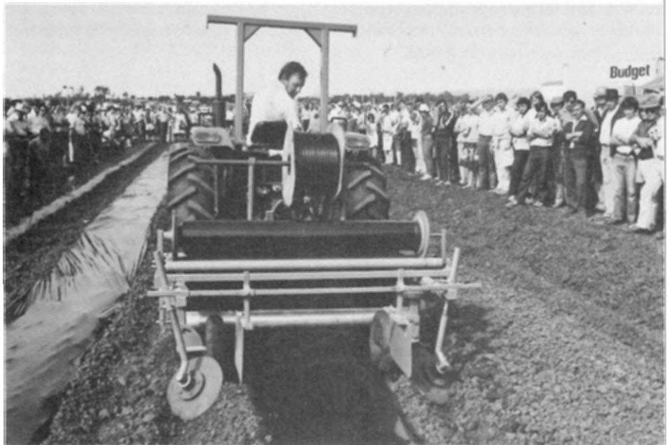
Bevan Zischke, a Departmental experimentalist at Bundaberg, demonstrates a machine that lays plastic mulch and trickle-irrigation hose for vegetable crops at the 1984 Horticultural Expo, held at Queensland Agricultural College.
