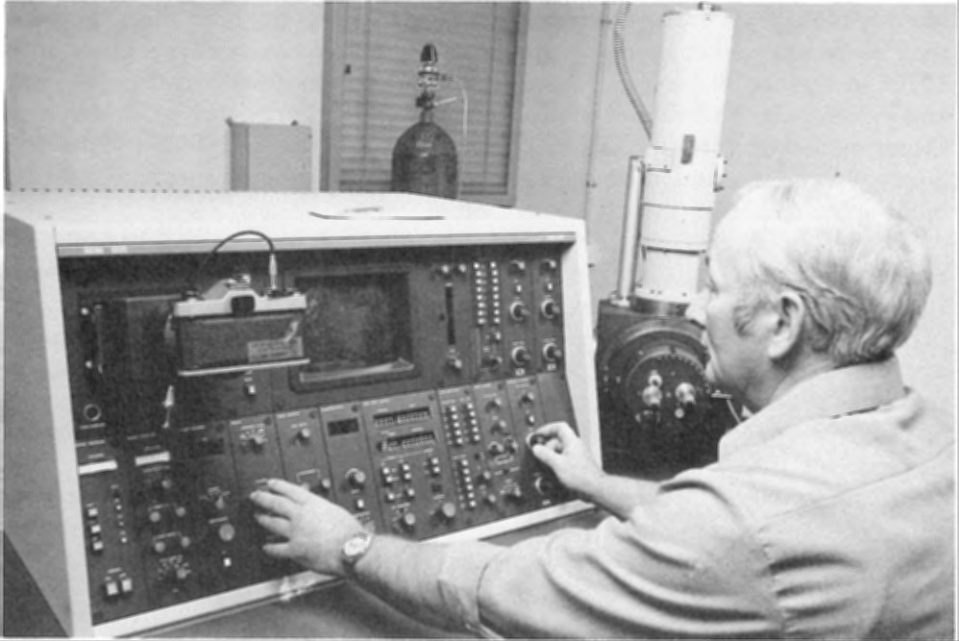
Don Gowanlock using the Philips 505 Scanning Electron Microscope, which was installed in the entomology laboratory at Indooroopilly in 1985 for plant and animal disease identification
