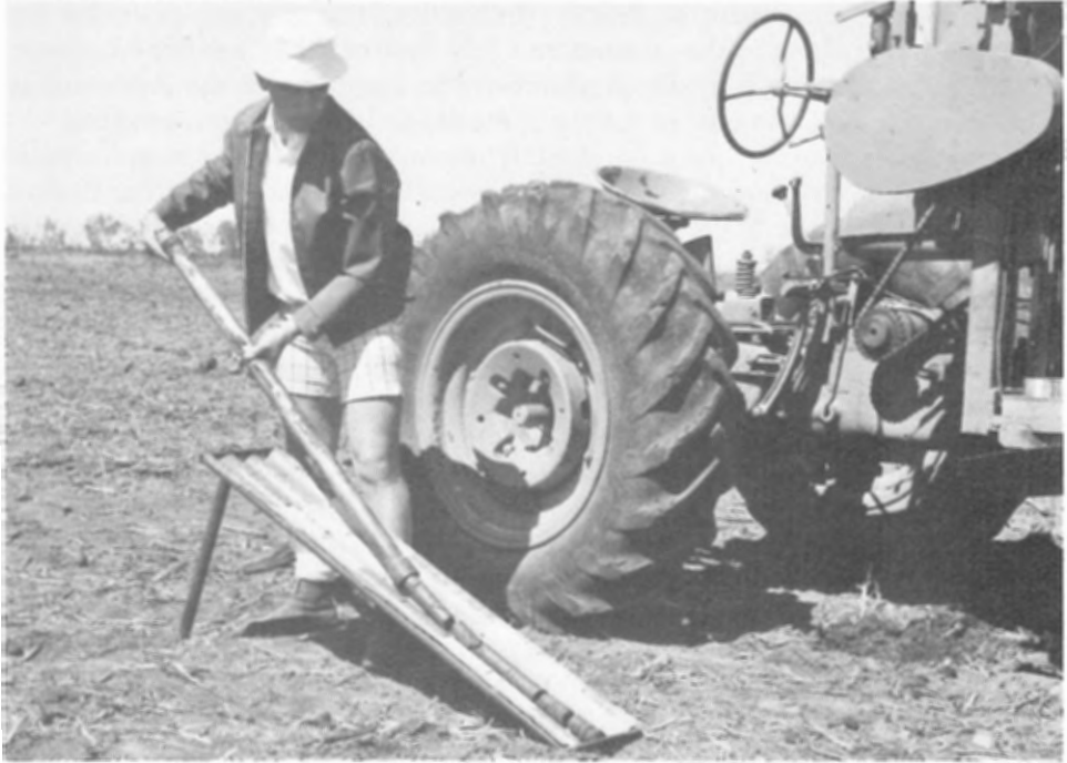
Brian Venz, an officer in the division of land utilisation, taking soil core samples at Brigalow Research Station in the early 1970s
