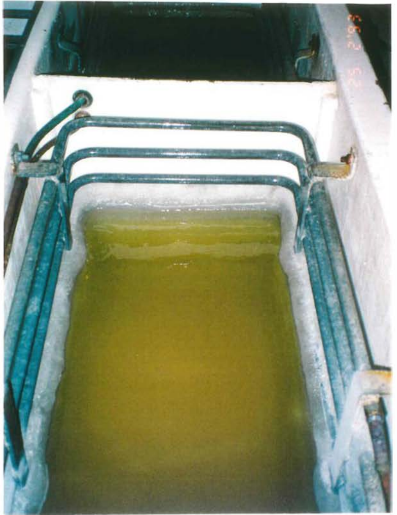
Figure 3.1 Contaminated refrigerated seawater used for storage of prawns
