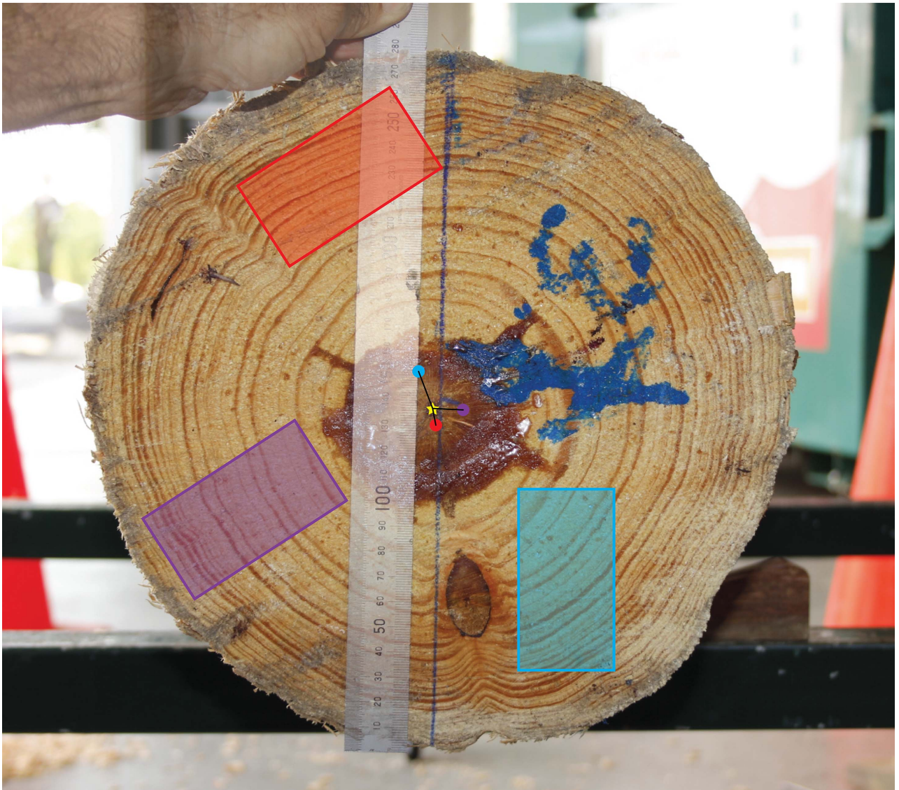
Fig. 1 The pith location algorithm tested on three sections of a swan log of radiata pine of approximately 28cm diameter. The coloured regions indicate the three different virtual cuts and the associated circle shows where the algorithm places the points where the yellow star is the true pith location. Image courtesy of Queensland Department of Agriculture and Fisheries (QDAF).
