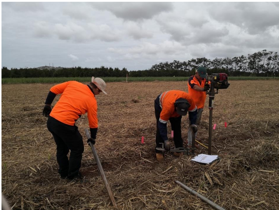
Figure 4. Deep soil sampling at Bundaberg after cane harvest.
