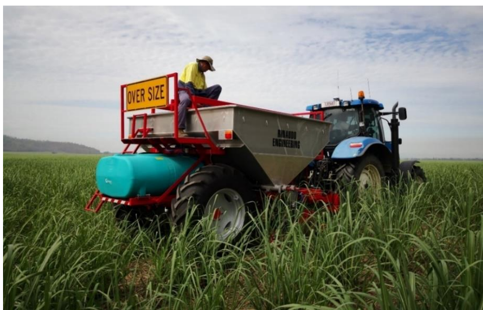
Figure 2. Application of nitrogen fertilisers in the experimental plots using a variable rate fertiliser applicator at the Lilypond site.
