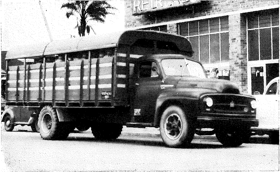
Fig. 5.—Vehicle C. Timber inserts fitted to conventional structure to restrict air movement to upper tier of cans.
