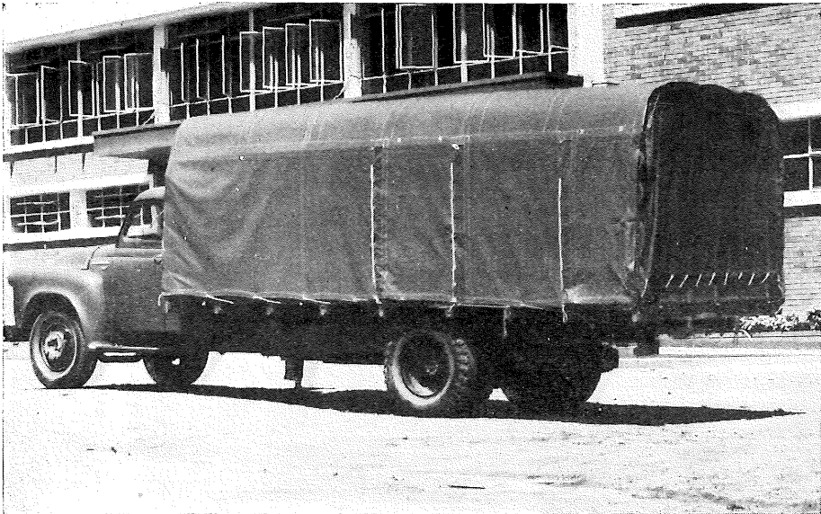
Fig. 2.—Vehicle A enclosed with a heavy-duty canvas canopy (Vehicle A1). Both front and rear ends are protected with separate flaps.
