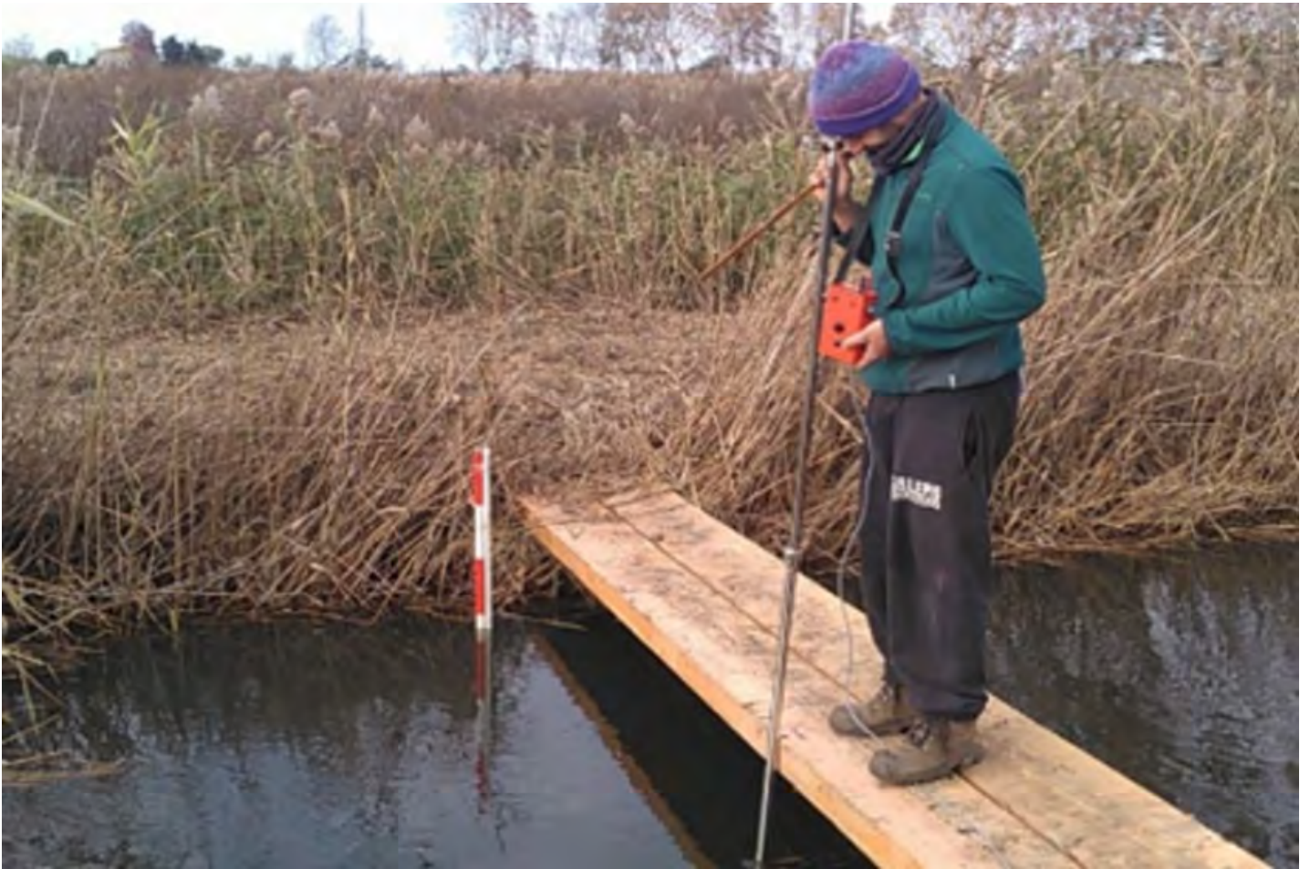
Figure 7: Detail of a gauging station to collect water level measurements using a water gauge and discharge measurements with a current meter Source: (Errico et al. 2019).
