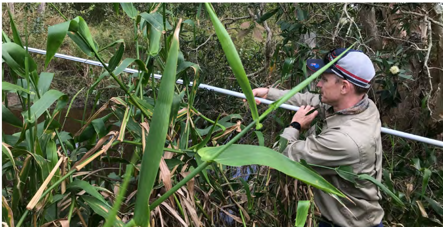
Figure 20: Using an extendable pole to collect water samples in a wetland.
