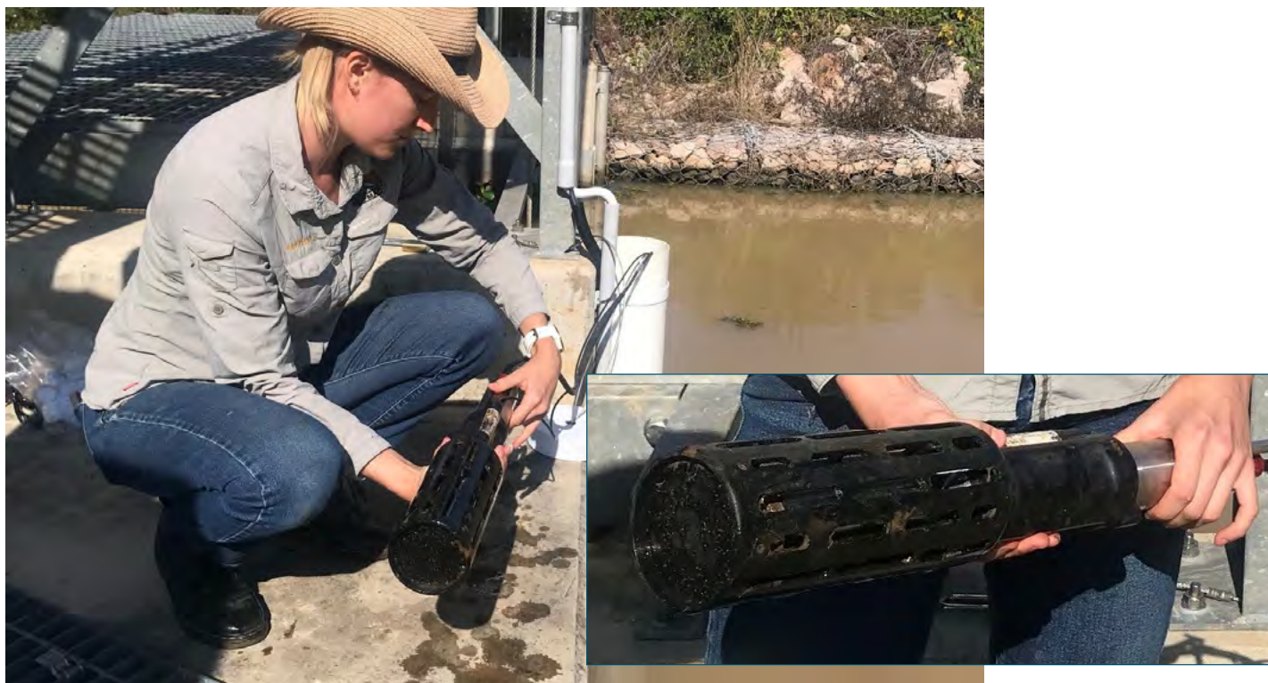
Figure 21: A nitrate probe set up to monitor catchment water quality. Inset shows a close-up of the nitrate probe with a screen to protect it from debris.
