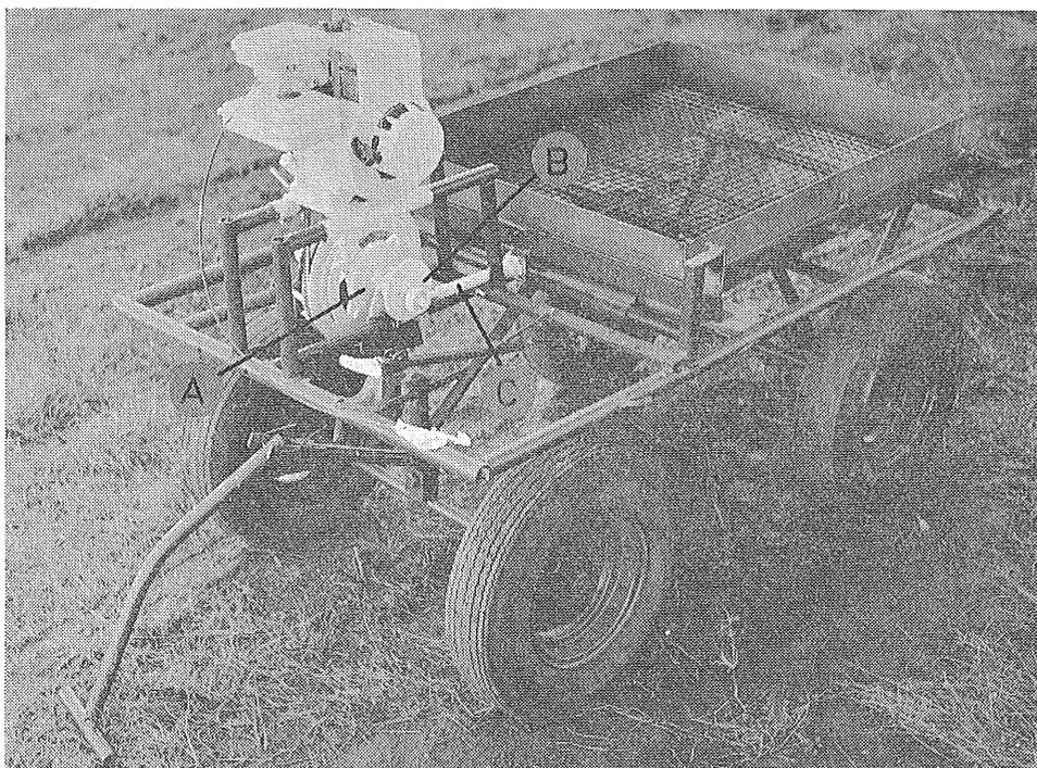
Plate 1.—The soil sieve fitted with one tray and mesh. A. Clutch B. Crank C. Connecting rod.
