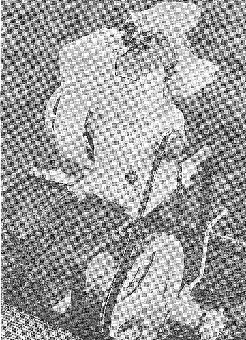
Plate 2.—Detail of motor and drive mechanism. A. Cam for engagement of clutch.
