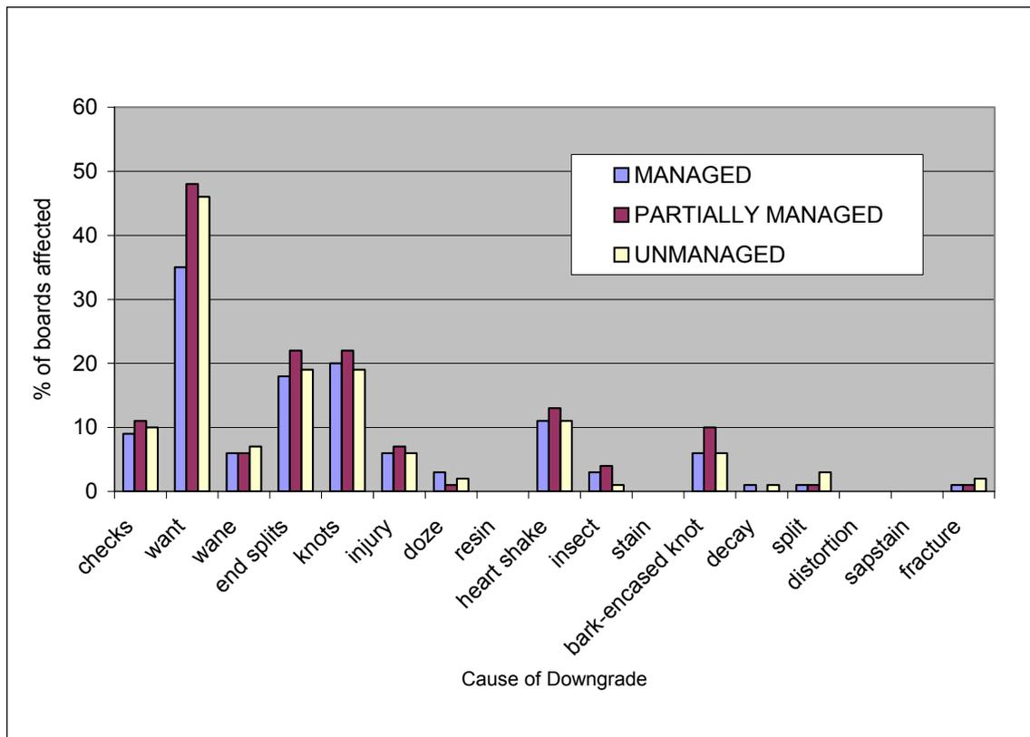
**Figure 32.** Percent of boards affected by defect type observed in boards from south west Queensland sites at the DGR stage.
