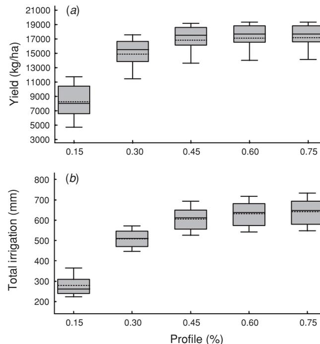
**Fig. 5.** The effects of starting soil water storage of 0.15 (15%) to 0.75 (75%) of capacity and refilling to these values, assuming no more than 60 mm of water deficit, and no less than 25 mm remaining in the profile on (a) predicted maize grain yield, and (b) amount of irrigation water (mm) used at Boort, Victoria, Australia, under non-limiting conditions of nitrogen supply using long-term weather data.
