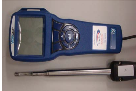
Figure 6. VelociCalc® 9545 air velocity meter. This unit has a range of 0-30m/s and can measure temperature and humidity
