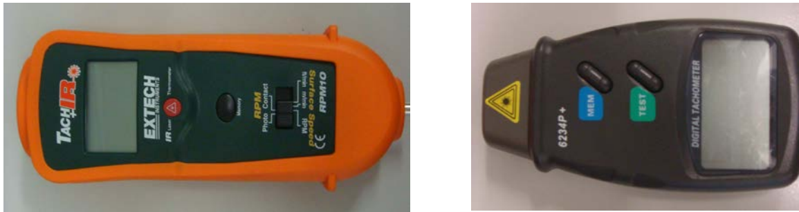
Figure 9. Digital tachometers used to measure fan rotational speed (rpm)
