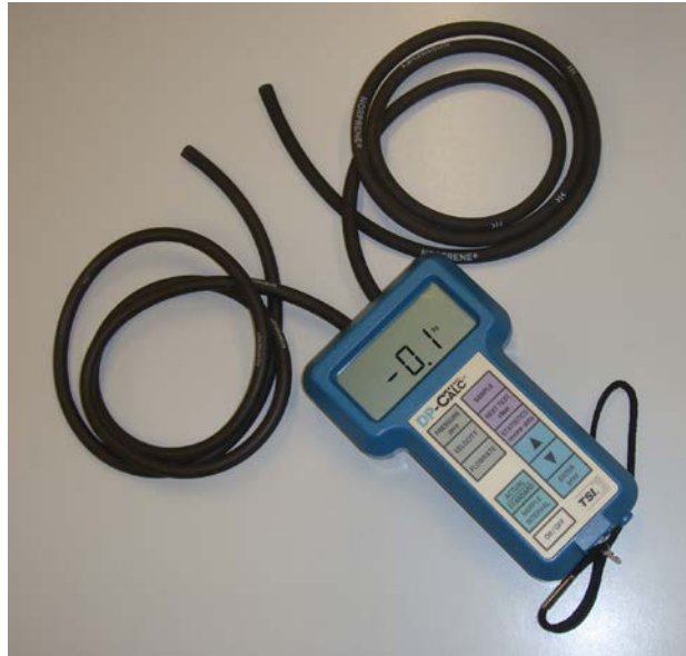
Figure 8. DP-Calc® 8705 differential pressure meter used to measure static pressure
