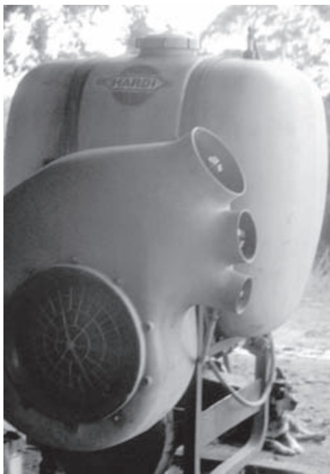
Figure 55. A typical three-point linkage air blast sprayer (top) another type of air blast sprayer (lower)
