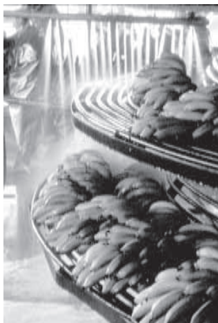
Figure 28. Washing bananas— by hand (upper); water spray over bananas on a packing wheel (lower)
