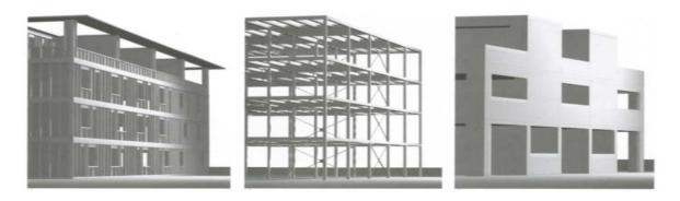
Lightweight Timber-Frame SystemsPost & BeamMassive Timber
