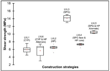
Figure 8.12. Shear strength results per construction lay-up type
