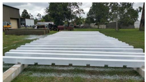
Figure 15.6. Painted veneer-based bridge kerbs
