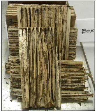
Figure 11.5. The majority of the pine feeder blocks were severely damaged by termites
