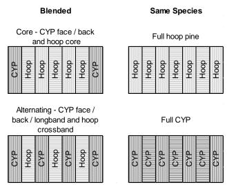
Figure 12.1. 7- ply plywood test block configurations (3 CYP thicknesses; 3 hoop pine thicknesses)
