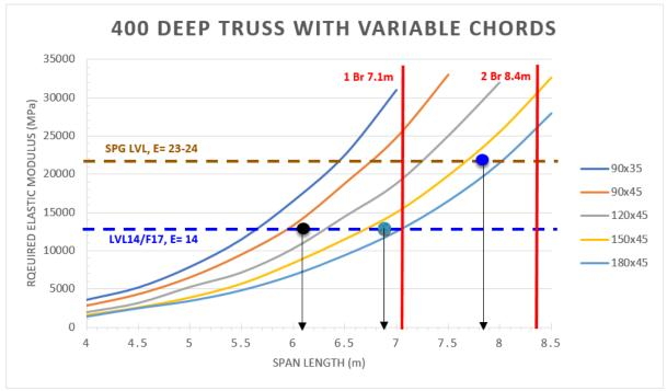
Figure 9.20. Comparison of spans for a 400mm deep floor truss with varying chord sizes and  ${\rm E}$
