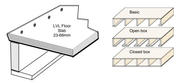
Figure 5.37. LVL Rib Slab – prefabricated floor cassette module options
