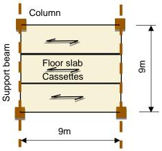
Figure 9.33. Typical office 9 x 9m grid
