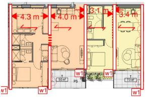
b) floor elements utilising internal LB walls
