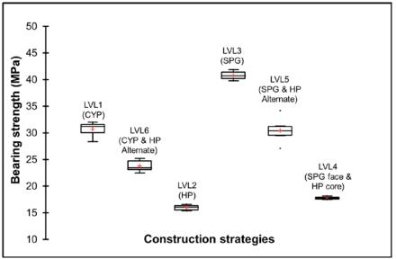
Figure 8.11. Bearing strength perpendicular to grain between investigated products
