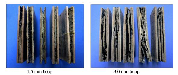
Figure 12.9. Extensive termite damage was sustained to the 1.5 and 3.0 mm hoop cores
