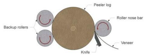
Figure 3.4. Spindleless lathe principles
