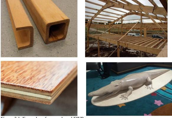
Figure 3.1. Examples of veneer-based EWPs
