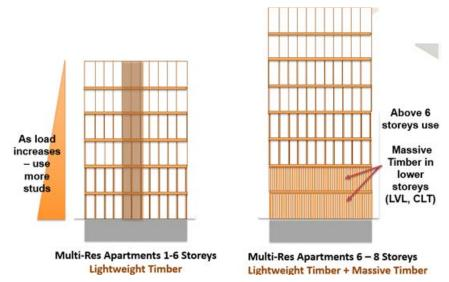
Figure 9.26. Lightweight timber framed mid-rise apartments
