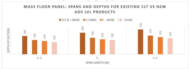
Figure 9.43. Floor panel depths of CLT and LVL of different E values for 5.0 and 5.5m spans
