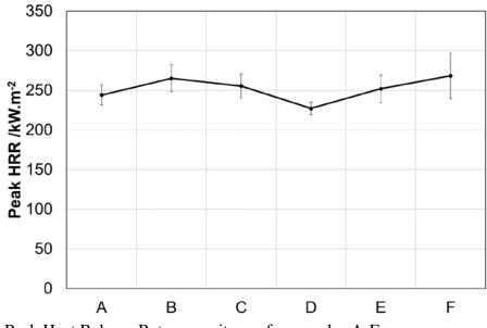
Figure 13.6. Peak Heat Release Rate per unit area for samples A-F.
