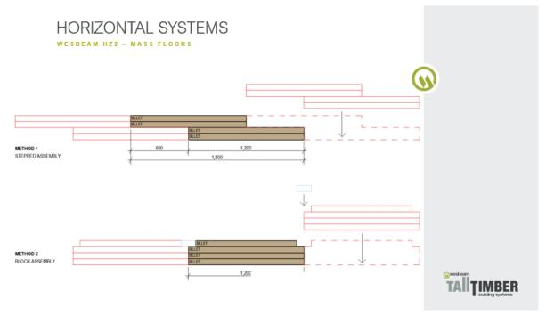
Figure 9.45. Possible joining arrangements for mass floor panels (image: David Bylund Wesbeam)
