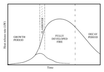
Figure 13.1. Classical temporal evolution of the heat release rate from the fire within a compartment.
