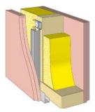
Figure 9.24. Single stud walls with resilient mounts
