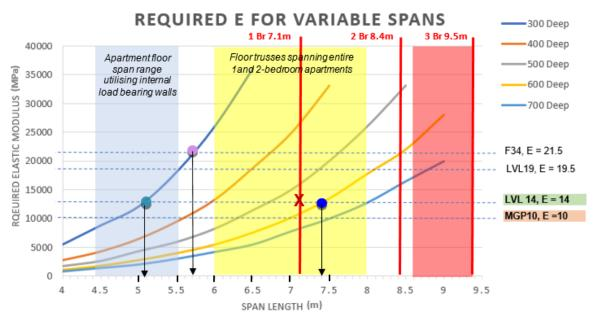
Figure 9.17. Spans for floor trusses of variable depth and E *Note: this assumes that the floor trusses are spaced at 450mm crs, the trusses utilise 90x45mm top and bottom chords.*
