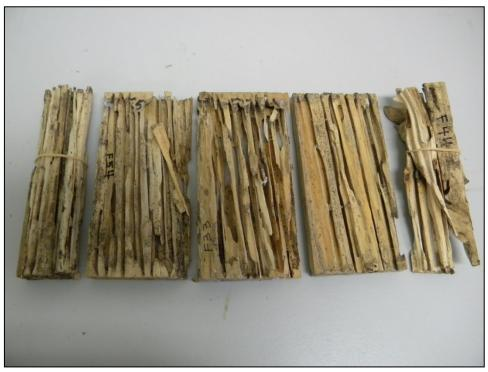
Figure 6.6. All pine sapwood blocks were severely damaged indicative of strong termite vigour
