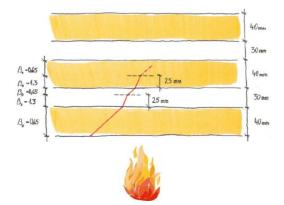
Figure 5.33. Change in Charring Rate with Polyurethane Adhesive (Stora Enso)
