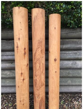
Figure 15.10. Proto-type bollards processed from white cypress pine
