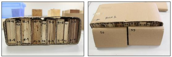
Figure 11.1. LVL test blocks and pine sapwood feeder blocks prior to placement in a termite exposure box
