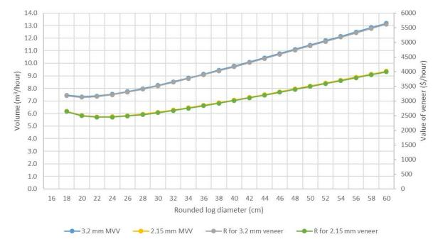
Figure 16.5. Volume and value per hour of 2.15 mm and 3.2 mm veneer produced from 2.6 m logs  $\,$
