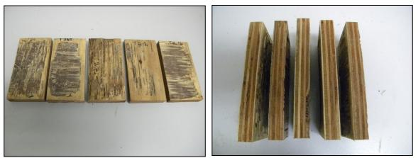
Figure 6.10. Configuration 2 plywood blocks had damage to the face and back veneers but inner plies were intact
