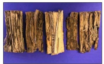
Figure 12.6. The majority of the softwood feeder blocks were substantially damaged by termites
