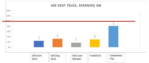
Figure 9.14 Floor truss design criterion comparison
