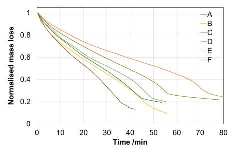
Figure 13.7. Normalised mass loss over time for samples A-F when exposed to 50 kW m<sup>-2</sup>.
