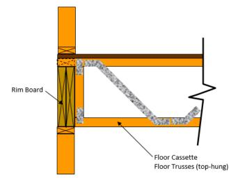
Figure 5.41. Use of a cassette floor with rim-board
