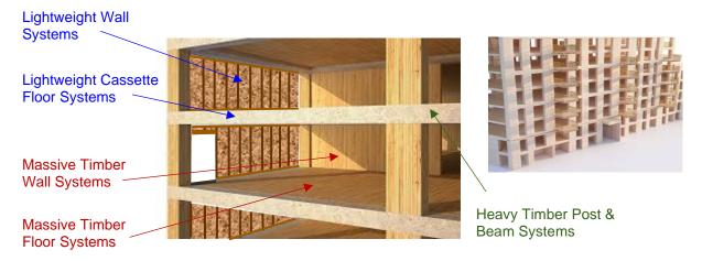
Figure 5.31. Timber based systems used in mid-rise timber buildings
