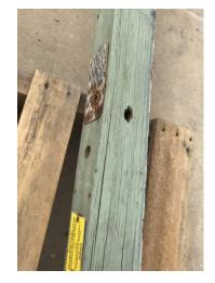
Figure 14.4. LVL cross-arm delamination
