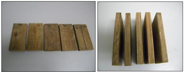
Figure 6.8. Configuration 4 plywood blocks had a visual rating of 1 and zero mass loss
