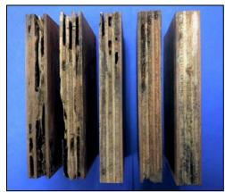
Figure 12.12. The 3mm hoop pine cross bands were badly damaged in some instances
