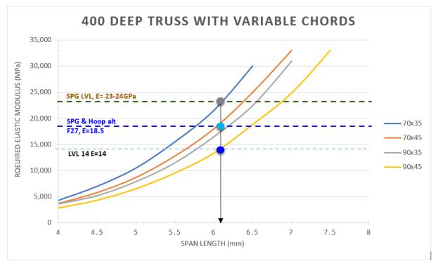
Figure 9.19. Effect of higher E grade materials on reduced cross section for a set span
