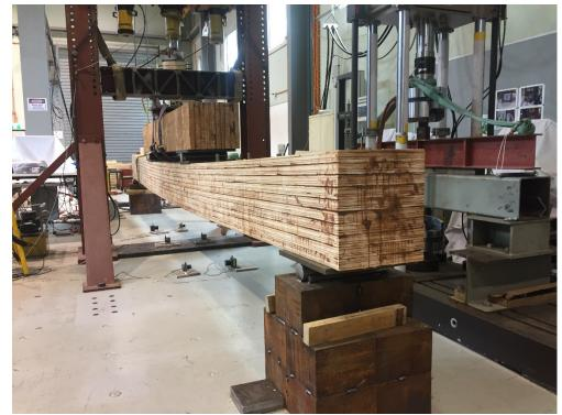
Figure 15.3. Strength testing of prototype veneer-based bridge girders
