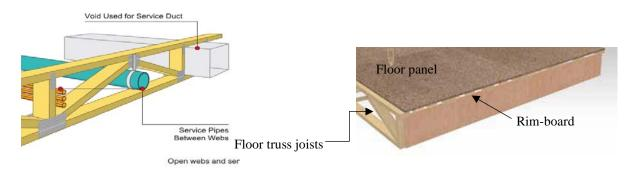
Figure 9.5. Openings in floor joist webs allow access for services
