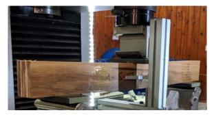
Figure 8.7. Testing configuration for longitudinal shear strength
