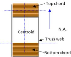
Figure 9.15. Floor truss elements
