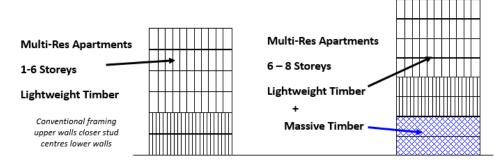
Figure 5.38. Wall framing approaches in 6-8 storey buildings
