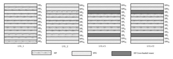
Figure 10.1. Construction strategies of LVL and LVL-C
