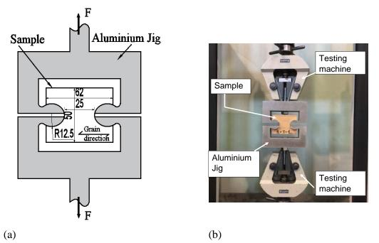
Figure 10.3. Tension perpendicular to grain test set-up, (a) schematic and (b) photo
