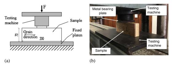
Figure 10.4. Compressive perpendicular to grain test set-up, (a) schematic and (b) photo
