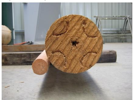
Figure 3.8. A 45 mm peeler core (left) produced from a spindleless veneer lathe compared with a 130 mm peeler core produced from a standard, commercial spindled lathe.
