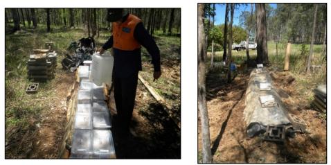
Figure 12.4. The exposure boxes were placed atop the trench and covered with black plastic
