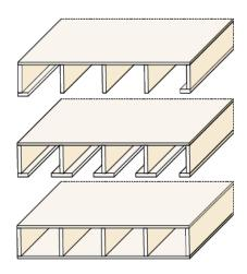
Figure 5.43. LVL floor slab configurations
