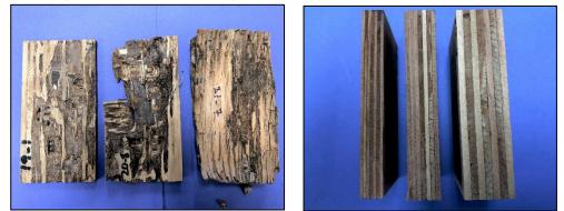
Figure 12.7. Hoop pine control blocks (L) were damaged by *C. acinaciformis* while CYP controls (R) didn't receive any damage
