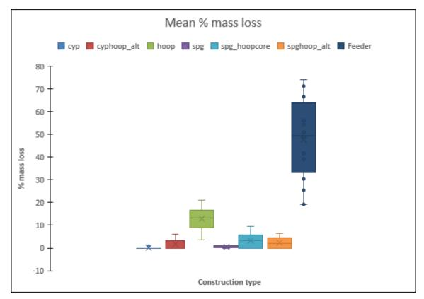
Figure 11.19. Mean % mass loss due to termite feeding per construction type including pine feeder
