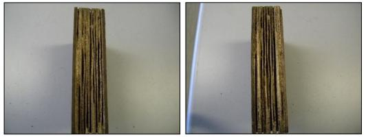
Figure 11.15. There was significant damage to the hoop core in some blocks
