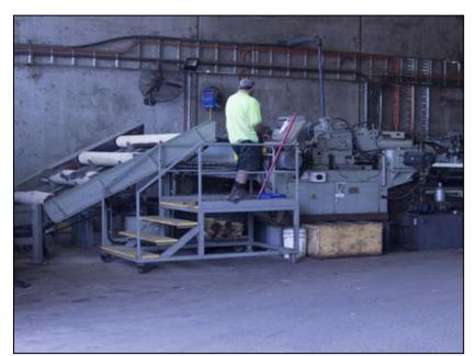
Figure 3.2. New commercial spindleless lathe operation in Australia
