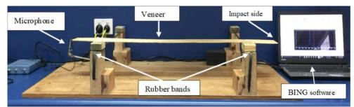
Figure 8.1. Experimental setup for the acoustic properties testing
