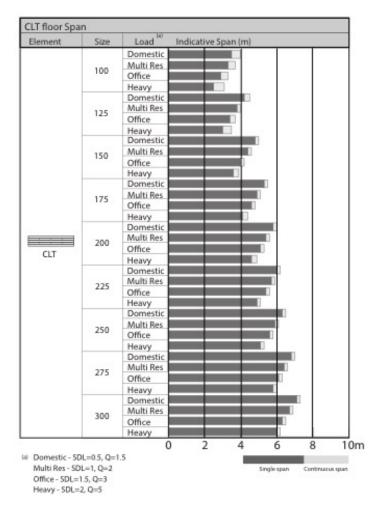
Figure 9.42. Indicative CLT floor panel spans - from WS Tech Guide #? 2018
