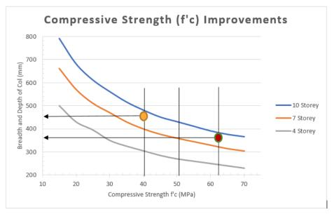
Figure 9.38. Square column dimensions with an improving compressive strength for a 4, 7 and 10-storey building with G = 2.8kPa and Q = 3kPa
