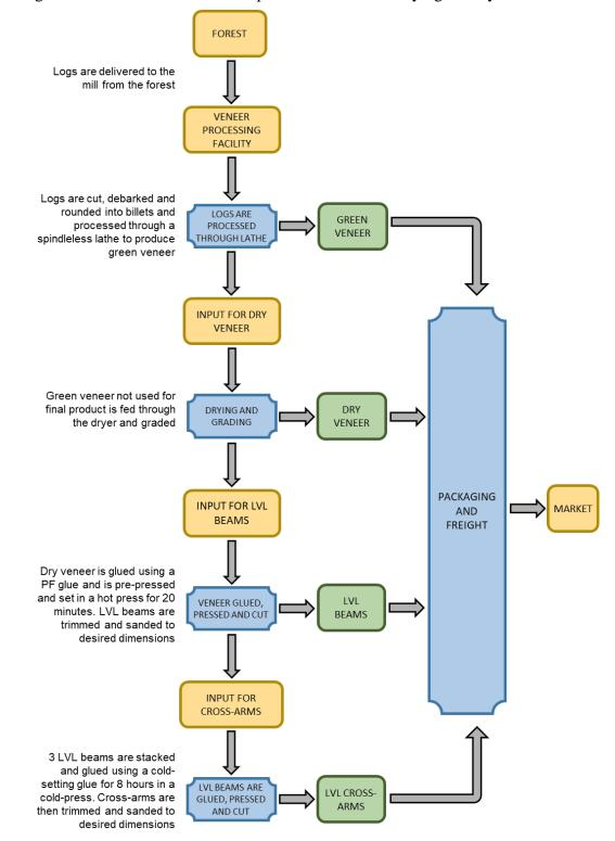
Figure 18.1. Schematic diagram of the evaluated veneer and EWP manufacturing process
