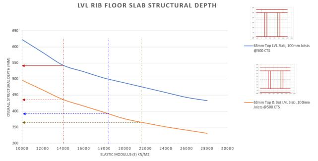
Figure 9.35. LVL rib-slab floors showing depth required for different modulus of elasticity material
