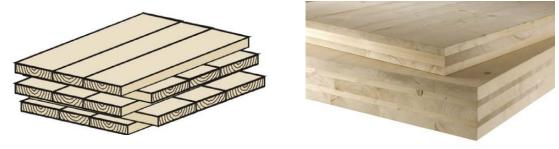
Figure 5.20. Cross-laminated timber
