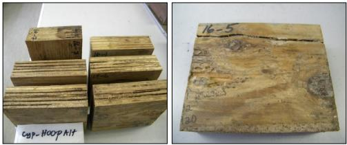
Figure 11.14. The cypress/hoop alt. LVL blocks sustained significant damage to some of the hoop plys
