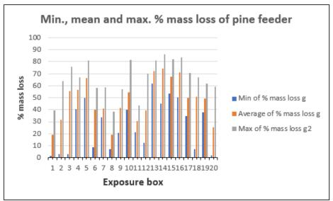
Figure 11.7. Minimum, mean and maximum % mass loss of pine feeder blocks per exposure box
