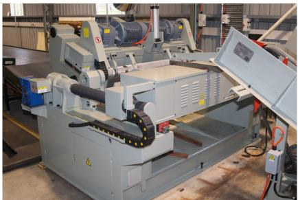
Figure 3.7. An example of a spindleless lathe
