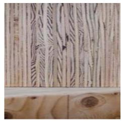
Figure 5.25. Veneer based mass panels
