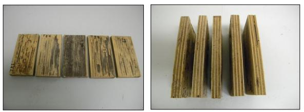
Figure 6.11. Configuration 3 plywood blocks had damage to the face and back veneers but the inner plies were intact
