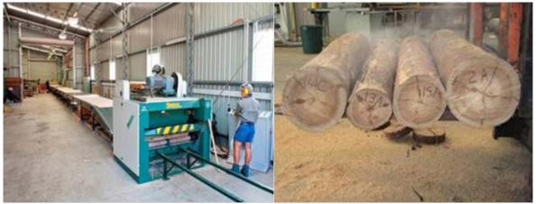
Figure 3.9. Spindleless lathe equipment and small-diameter peeler billets at the Wood Composites Facility, DAF Salisbury Research Facility
