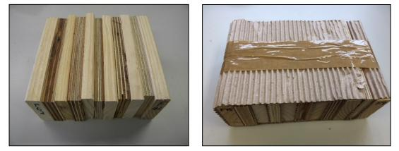
Figure 6.1. Plywood blocks and pine sapwood blocks prior to placement in termite exposure box
