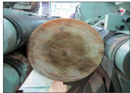
Figure 3.3. A small-diameter hardwood log being peeled with a spindleless lathe
