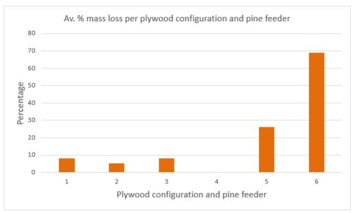
Figure 6.12. Average percentage mass loss due to termite feeding for five plywood configurations plus pine feeder
