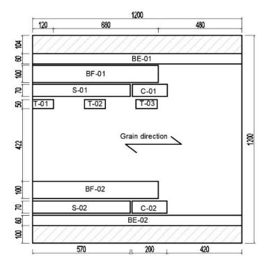
Figure 8.3. The cutting pattern for the LVL for property tests *Note:* BE – edgewise bending tests, BF – flatwise bending tests, S – longitudinal-tangential shear bending tests, C – compression perpendicular to the grain tests, T – tension perpendicular to the grain tests.
