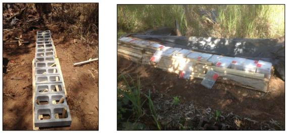
Figure 6.2. Exposure boxes placed on concrete blocks atop a termite aggregation trench at Esk
