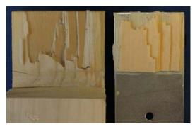
Figure 5.46. Embedded steel connection reinforcement plates
