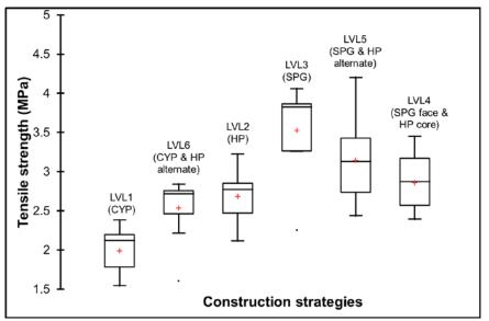
Figure 8.10. Comparison of tension strength perpendicular to the grain for all the investigated products
