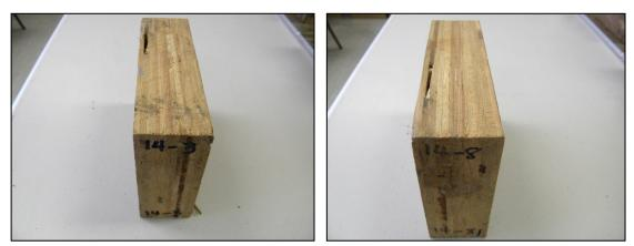
Figure 11.11. Two of the 100% cypress LVL blocks sustained minor damage to one of the inner plys
