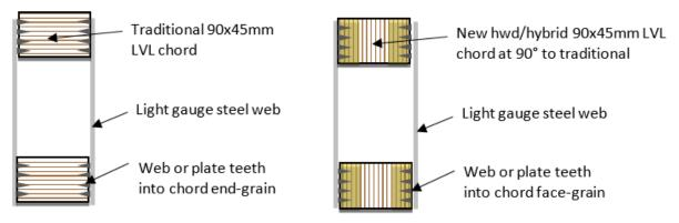
Figure 9.21. Floor truss chord orientation configurations
