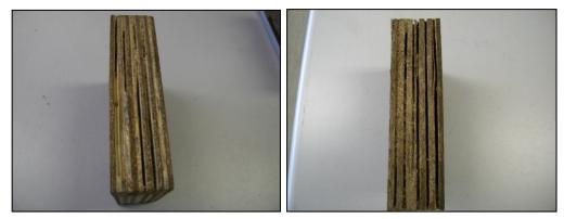
Figure 11.16. There was significant damage to the hoop plys in some of the blocks
