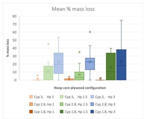
Figure 12.10. Mass loss % of nine plywood configurations comprising a CYP face and back and a hoop pine core (cross is the mean; central horizontal bar is the median)
