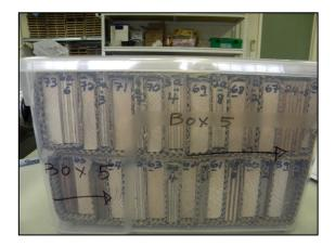
Figure 12.2. Plywood test blocks and pine feeder sapwood blocks positioned in an exposure box
