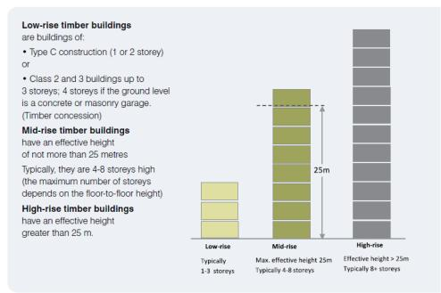
Figure 5.30. Terminology for different timber construction options
