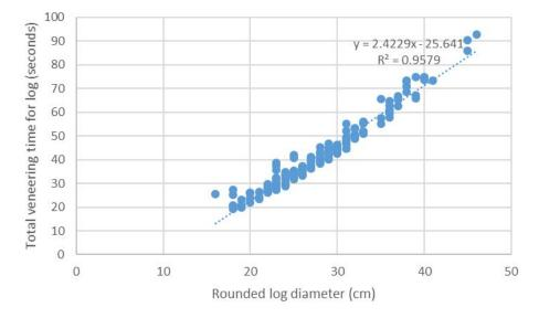
Figure 16.4. Total veneering time by rounded log diameter for 3.2 mm thick veneer peeled at 40 lm per minute
