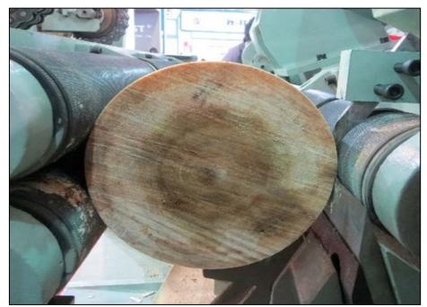
Figure 2.2. A small-diameter hardwood log being peeled with a spindleless lathe.
