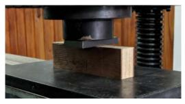
Figure 8.5. Testing configuration for bearing strength perpendicular to the grain
