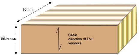
Figure 9.31. Possible new hardwood LVL/MPP product with grain orientated at 90 degrees
