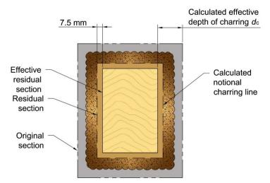
Figure 9.40 Loss of section due to charring
