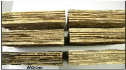
Figure 11.8. Fifteen of the 100% hoop pine LVL blocks were severely damaged by *C. acinaciformis*
