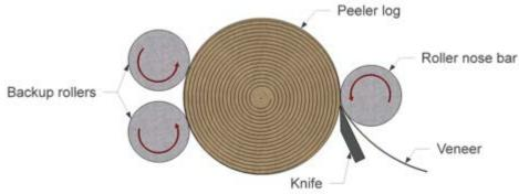
Figure 2.3. Spindleless lathe principles
