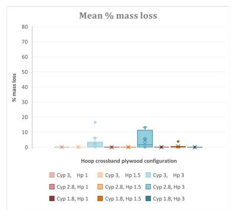
Figure 12.13. Mass loss % of nine plywood configurations comprising a CYP face, back and long band and a hoop pine cross band (cross is the mean; central horizontal bar is the median)
