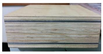
Figure 5.47. Steel reinforced plywood doors for prisons (Big River)
