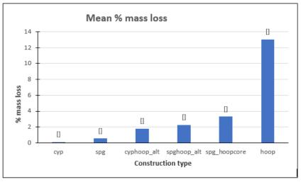
Figure 11.20. Mean % mass loss due to termite feeding per construction type
