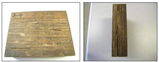
Figure 11.13. Block 3\_4 sustained damage to the face and back veneer and inner ply with a visual rating of 3
