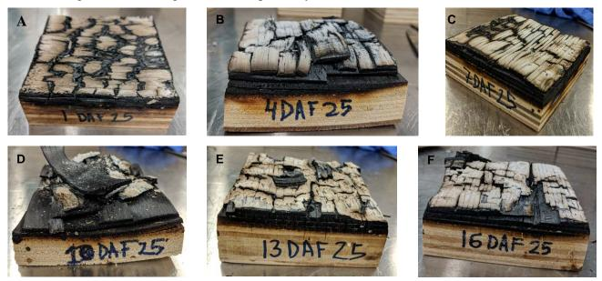
Figure 13.9. Samples A-F after exposure to 25 kW m<sup>-2</sup>.
