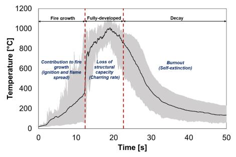
Figure 13.2. Performance criteria for each the stages of the fire. Heat release rate obtained from a full-scale CLT compartment fire test developed by The University of Queensland.
