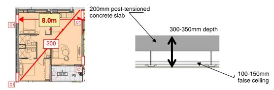
Figure 9.10. Typical post-tensioned concrete construction
