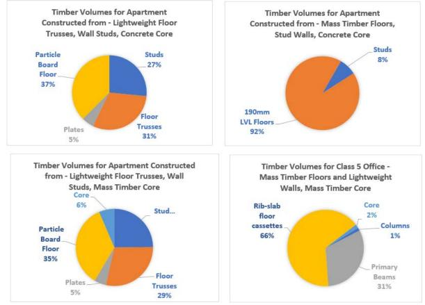
Figure 9.49. Total volume of timber by percentage for each construction methodology
