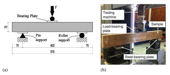
Figure 10.5. Longitudinal-tangential shear test set-up, (a) schematic and (b) photo
