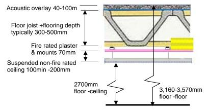
Figure 9.8. Typical mid-rise floor system build-up
