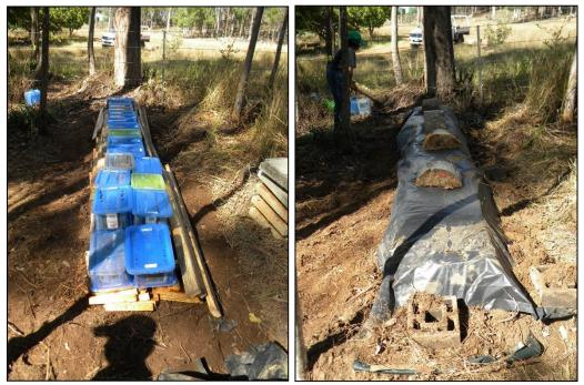
Figure 11.3. The exposure boxes were placed atop the aggregation trench and covered with black plastic
