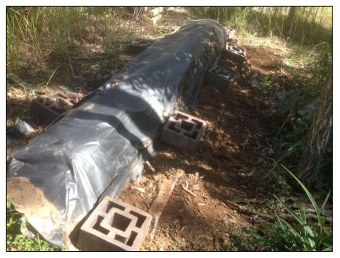
Figure 6.3. The exposure boxes were covered to provide a dark, humid foraging environment
