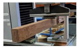
Figure 8.4. Testing configuration for flatwise (left) and edgewise bending (right)
