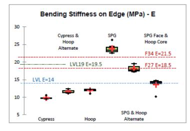
Figure 9.32. Initial prototype LVL testing results for MoE
