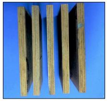
Figure 12.11. Test blocks with a CYP long band and a 1.0 mm hoop pine cross band were undamaged
