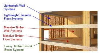
Figure 9.2. Typical timber-based systems used in mid-rise timber buildings
