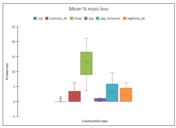
Figure 11.18. Mean % mass loss due to termite feeding per construction type
