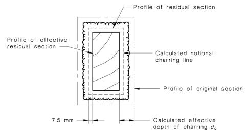
Figure 5.32. Loss of section due to charring
