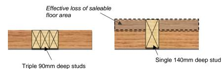
Figure 9.25. Using multiple smaller width stud instead of a deeper stud
