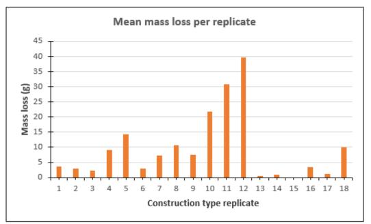
Figure 11.22. Mean percentage mass loss per replicate per construction type *Note:*
