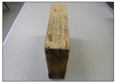
Figure 11.9. Block 10\_4 was the least damaged of all the 100% hoop pine LVL blocks
