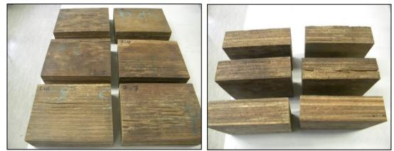
Figure 11.12. Fifteen of the 100% SPG blocks had minor damage to the face and/or back veneers and inner plys
