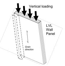
Figure 5.45. Massive LVL wall
