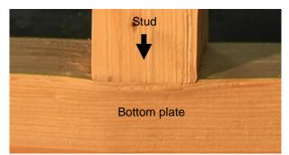
Figure 9.29. Illustration of perpendicular to grain crushing of bottom plate due to stud
