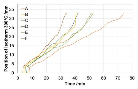
Figure 13.8. Position of the isotherm 300°C over time for sample A-F when exposed to 50 kW m<sup>-2</sup>.
