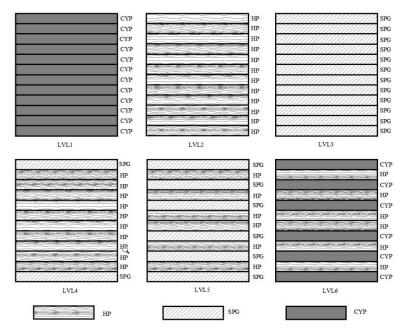
Figure 8.2. LVL panel construction lay-up types
