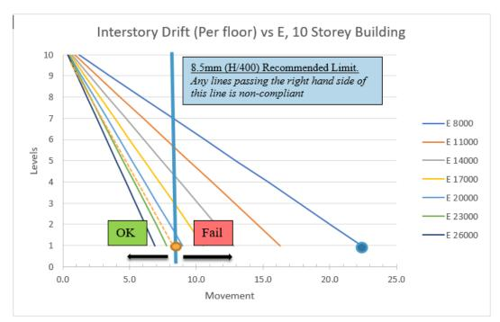
Figure 9.47. 'Back of the envelope calculation' indicating the improvements for an increasing elastic modulus
