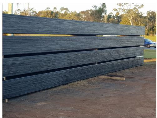
Figure 15.4. Veneer-based bridge girders ready for dispatch
