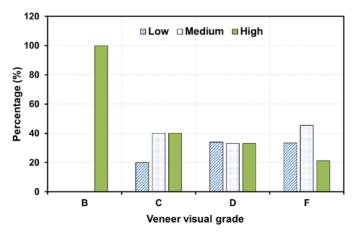
Figure 10.7. Correlation between visual grading and MOE grading of SPG veneers
