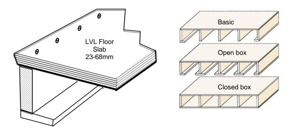
Figure 9.34. LVL Rib-Slab floor cassette module options
