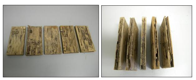
Figure 6.7. All control plywood blocks sustained damage to face and back veneers and inner plies
