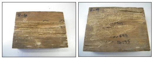
Figure 11.17. Two blocks sustained significant damage to the face veneer
