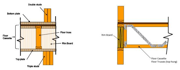
Figure 5.44. Wall and floor cassette products needing superior compression parallel to grain performance
