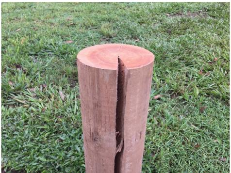
Figure 15.9. An extreme example of severe heart shakes caused during post-processing drying
