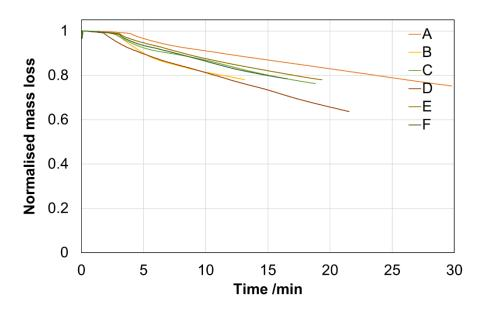
Figure 13.10. Normalised mass loss over time for samples A-F when exposed to 25 kW m<sup>-2</sup>.
