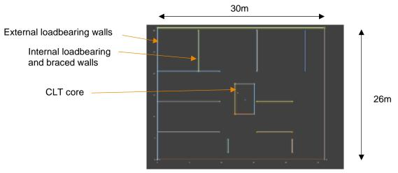
Figure 9.27. Analysis apartment plan of load bearing and bracing walls
