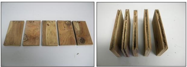
Figure 6.9. Configuration 1 plywood blocks had no damage to the face or back veneers but inner plies were eaten
