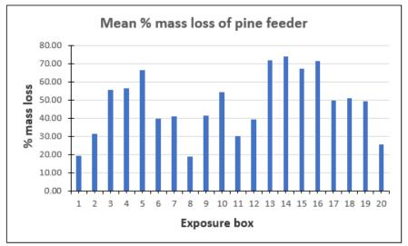
Figure 11.6. Mean % mass loss of pine feeder blocks per exposure box
