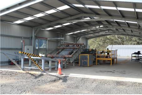
Figure 15.7. A newly installed spindleless debarker for the production of posts and bollards
