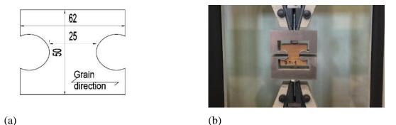
Figure 8.6. Testing configuration for tensile strength perpendicular to the grain
