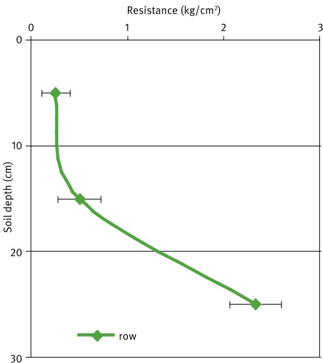
**Figure 22. Soil resistance is greater in wheel tracks than row area down a soil profile to 30 cm (top graph). The shape of the resistance curve is important, a sharp increase in the resistance reading can show a subsurface compaction layer (bottom graph)**
