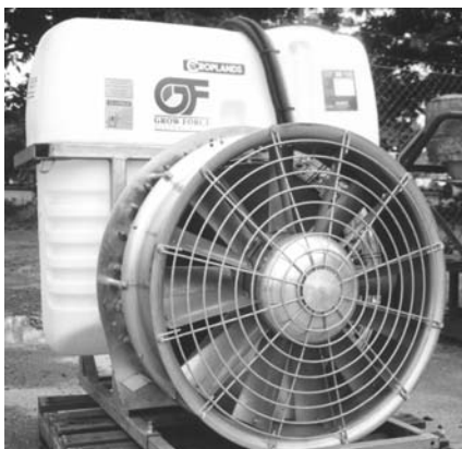
Figure 30. A typical three-point linkage air blast sprayer
