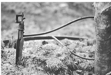
Figure 23. An under-tree minisprinkler
