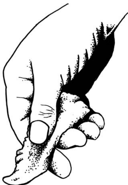
Figure 3. Ribbon test for assessing soil texture
