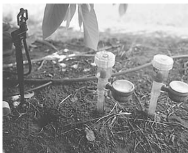
Figure 25. Tensiometers in place, (a) in major root zone and (b) below most roots
