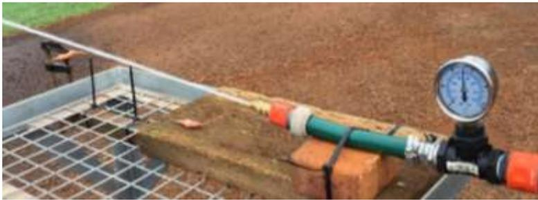
Figure 1: Hydraulic periderm removal apparatus, experiment 1, 50 DAP.
