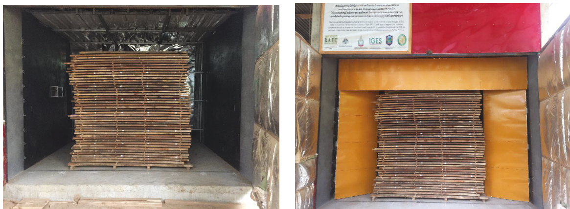
Figure 16: Installation of baffling in Mr Niphone’s kiln in Luang Prabang (left: before baffles were installed, right: timber stack with baffles installed)
