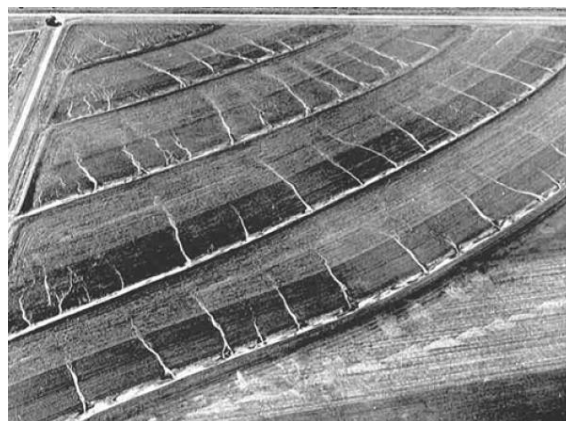
Figure 2. Cascading contour bank failure on a 6% slope, with 60m contour bank spacing (Thomas et al. , 2007)
