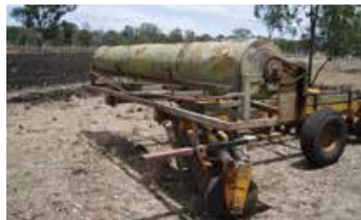
Roller or drum seeders are necessary to sow uncoated, fluffy grass seeds such as Rhodes grass and bluegrasses.
