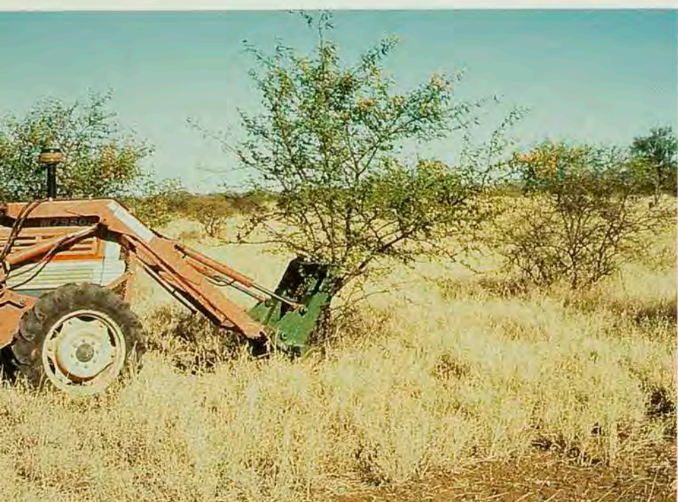
The grubber blade is especially useful for scattered prickly acacia bushes
