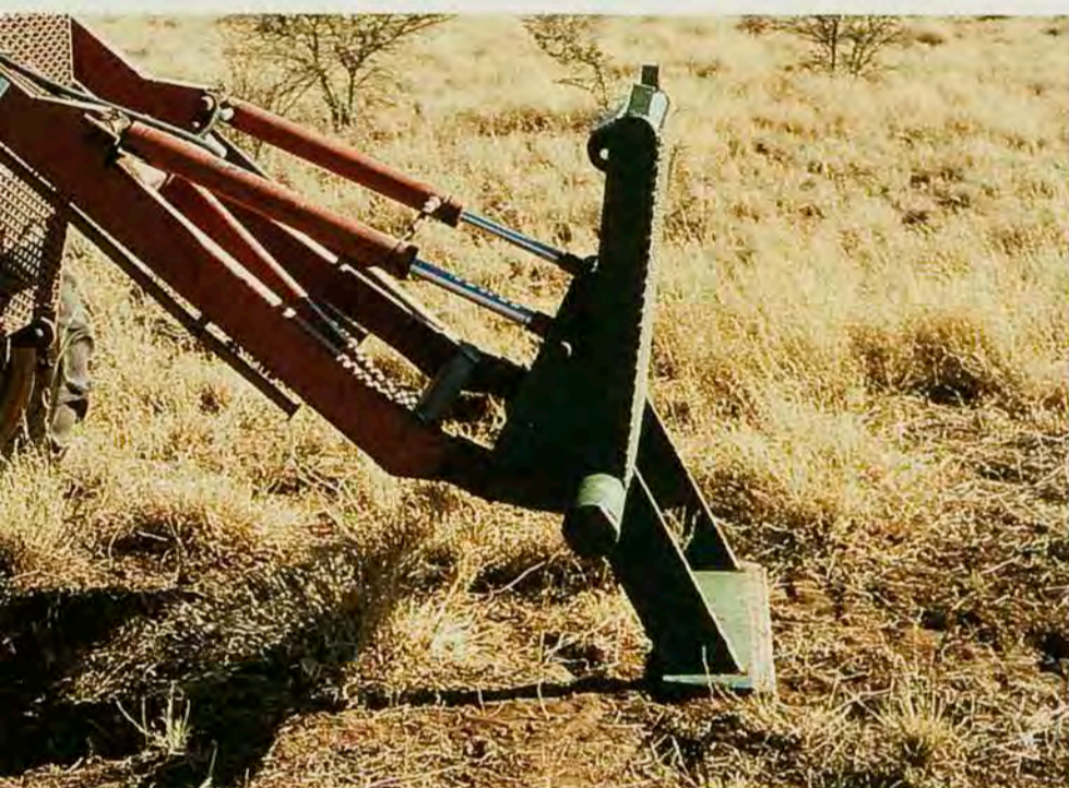
Grubber blade mounted on front-end loader
