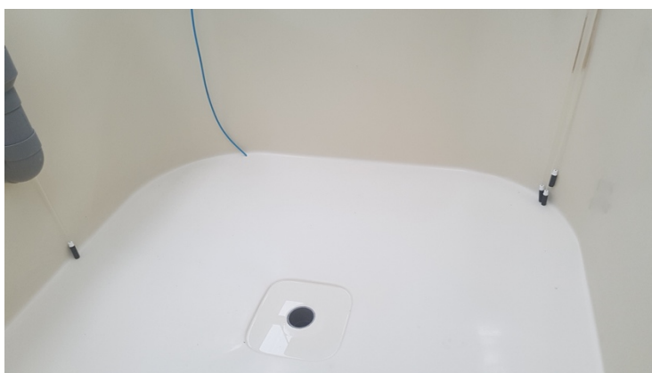
Figure 14: Culture tank with air diffusers
