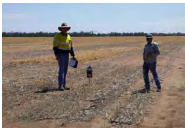
Taking monthly neutron moisture meter readings.
