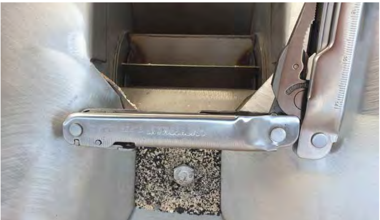
Figure 2. Metering unit for amendment application, with ruler for scale.
