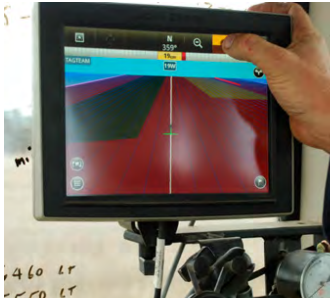
FIGURE 2-14 (f). The grower has pre-mapped this paddock for soil pH and is using GPS and variable rate technology to apply granular inoculant at higher rates on the low pH areas of the paddock and lower rates on the neutral areas.
