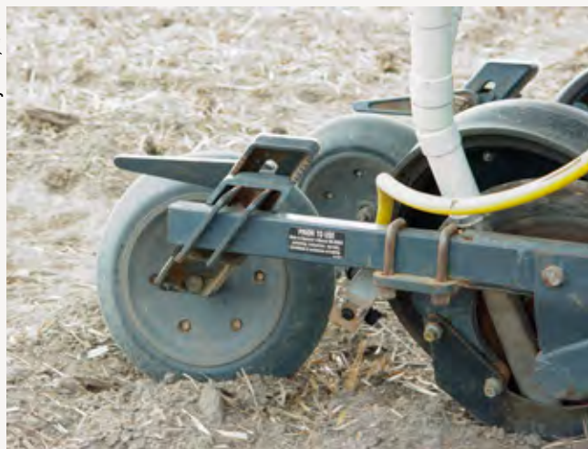
FIGURE 2-13 (a). Spray line attached behind planting tyne/boot used to disperse inoculants into furrow (water injection).
