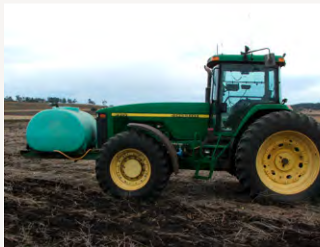
FIGURE 2-13 (b). Water tank mounted on tractor to apply inoculants by water injection.
