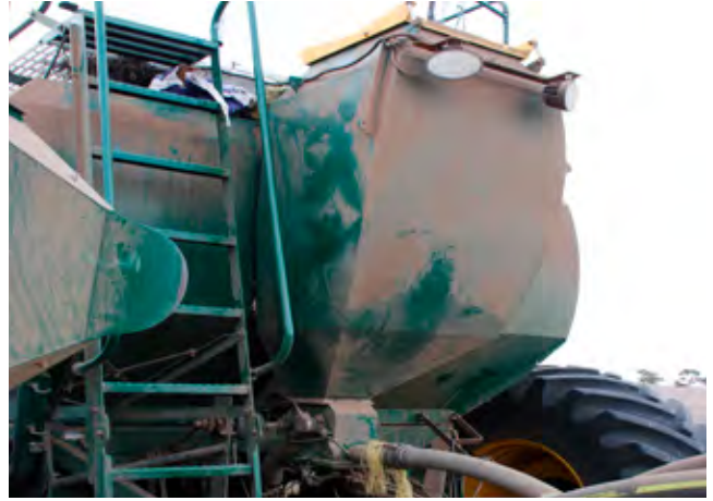
FIGURE 2-14 (b). Third box on the back of the seeder containing granular inoculant.
