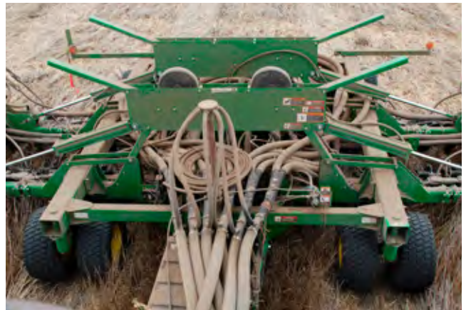
FIGURE 2-14 (d). For this air-seeder the seed, fertiliser and granules are mixed together in the air flow just prior to delivery to the soil furrow.
