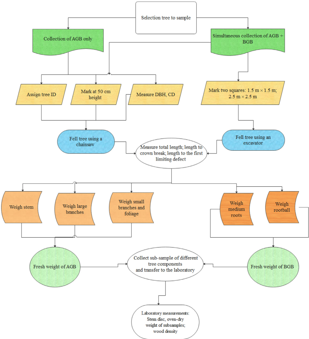
Fig. 2. Diagram of fundamental steps to collect AGB and BGB in the field.
