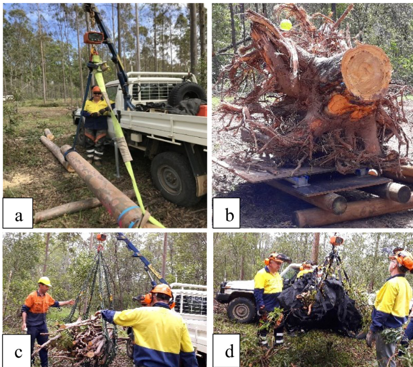
Fig. 4. Weighing tree components in the field to obtain fresh weight: (a) 3.0 m section of the main stem measured using digital crane scales lifted using a Hiab, (b) rootball measured on cattle scales, (c) large branches, and (d) small branches and foliage lifted in a cargo net using the Hiab and digital crane scale.
