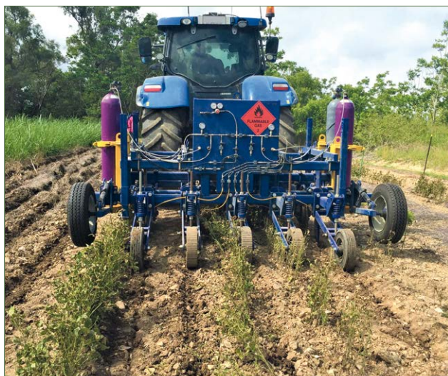
A tractor-mounted ethylene-injection system used to accelerate depletion of the soil seed-bank of red witchweed
