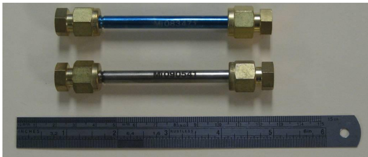
Figure 11: An example of two sorbent tubes with brass caps—the upper tube is coated in an inert coating to prevent oxidation of highly volatile species during sampling
