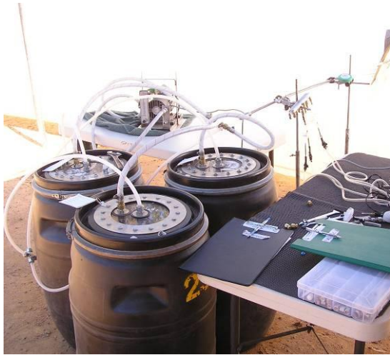
Figure 7: Odour sample collection from the polyethylene duct in Queensland
