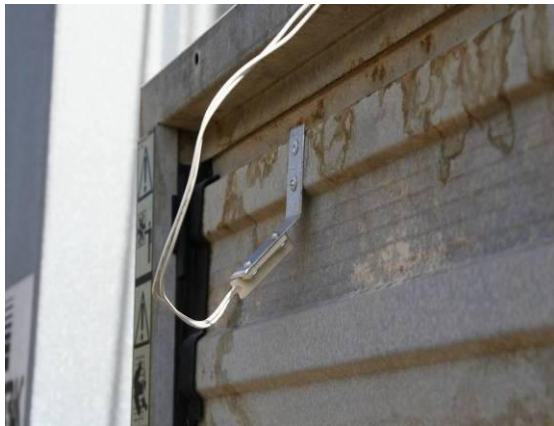
Figure 20: Mercury tilt switch with fan turned off (shutters closed, switch closed)
