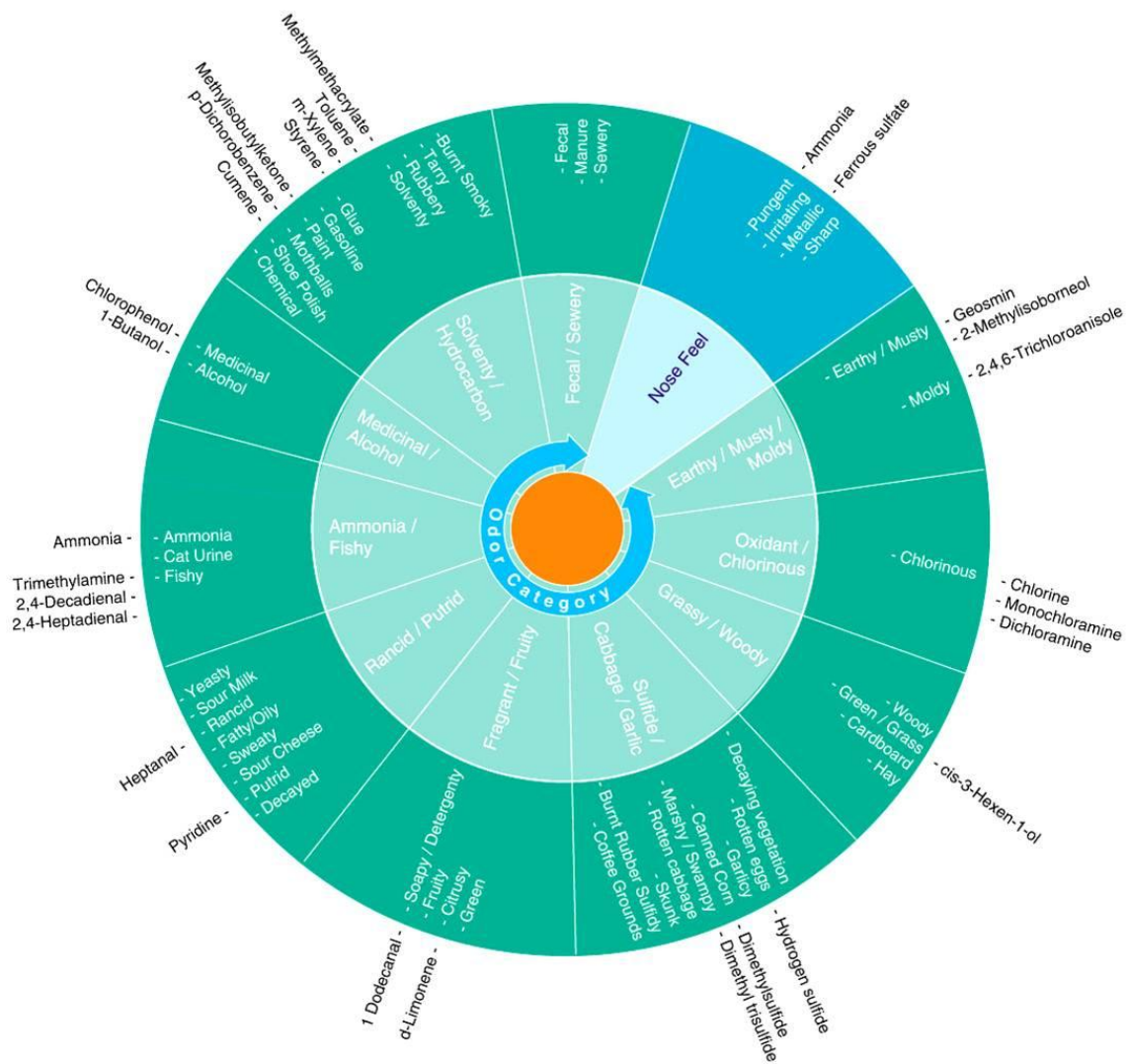
Figure 4: Taste and odour wheel for off-flavours in drinking water (Suffet et al. , 1999) showing the highlighted relationship between earthy – musty odours and compounds, geosmin and MIB (2-Methylisoborneol)
