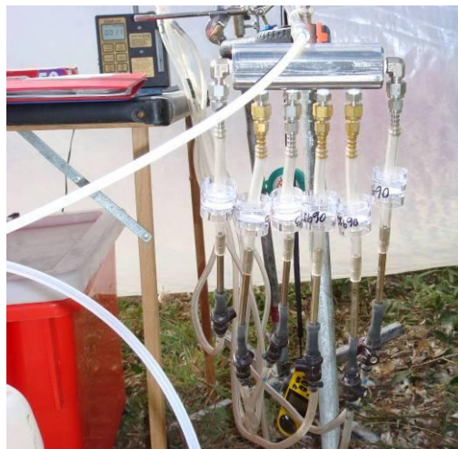
Figure 14: Filtered VOC tubes and manifold
