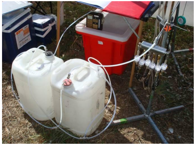
Figure 8: Odour sample collection from the polyethylene duct in Victoria
