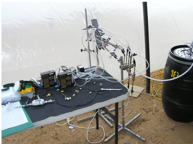
Figure 13: VOC sampling from duct
