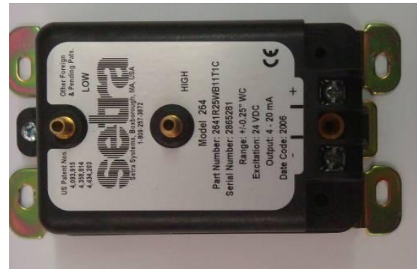
Figure 23: Setra ultra low differential pressure transducer used to measure the shed static pressure
