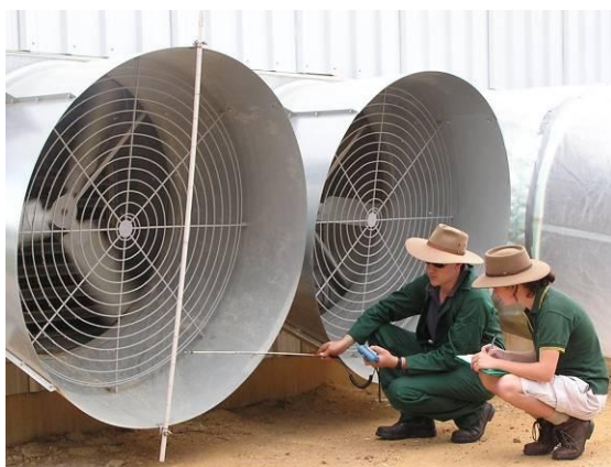
Figure 17: Measurement of airspeed at fan face (External)
