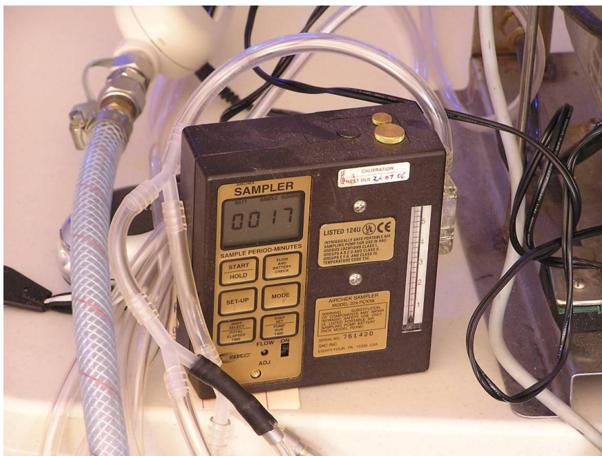
Figure 12: Vacuum pump used to draw the air samples through the sorbent tubes to collect the analytes
