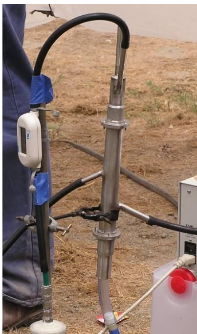
Figure 9: Isokinetic sampler used for particulate measurement
