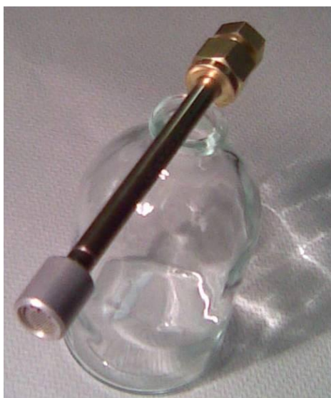
Figure 15: Sorbent tube with diffusion cap in place
