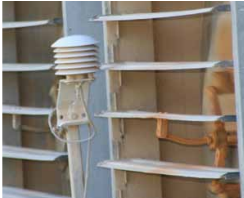
Figure 14: Radiation shield used at the exhaust fan (to measure shed emission temperature) and on the weather station
