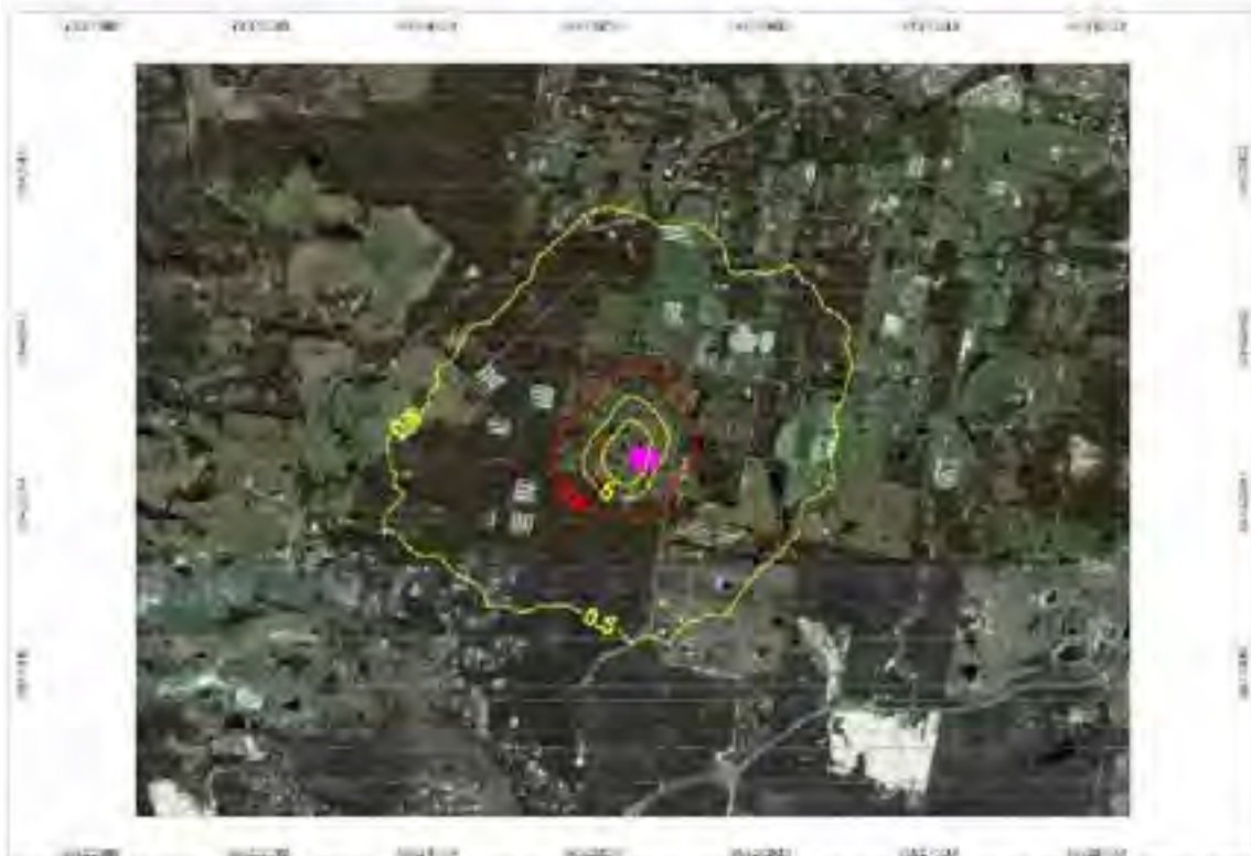
Figure 5.6: Predicted 99.5 th percentile odour concentrations for Case 3, four poultry shed scenario (OU)
