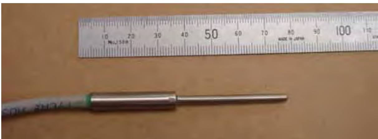
Figure 12: Platinum RTD (PT100 sensor inside a thin stainless steel sheath)
