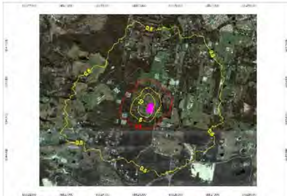
Figure 5.7: Predicted 99.5 th percentile odour concentrations for Case 3, eight poultry shed scenario (OU)
