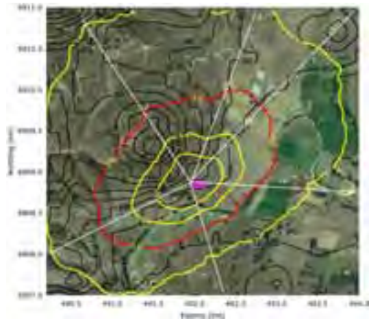
Appendix 9 Figure 19: 4 sheds ambient emission temperature
