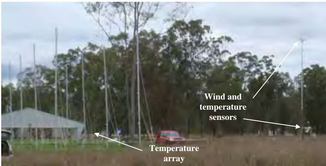
Figure 21: Weather station used for this project: temperature array in the background
