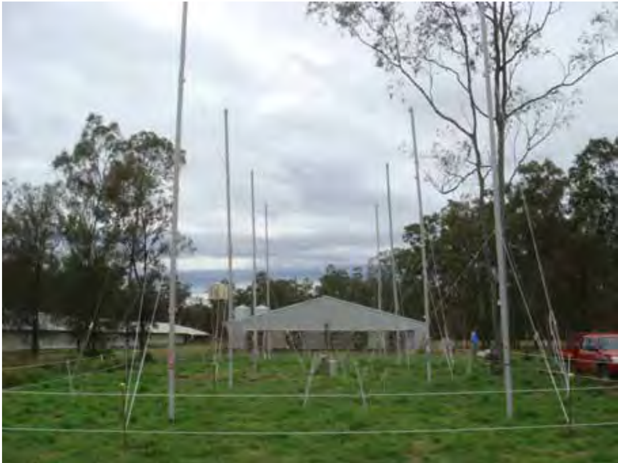
Figure 11: Temperature sensor array as installed at the broiler farm
