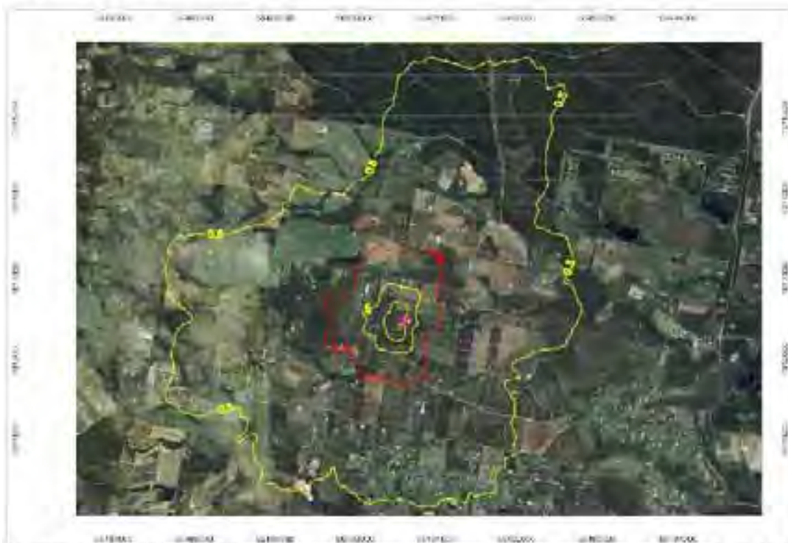
Figure 4.8: Predicted 99.5 th percentile odour concentrations for Case 2, four poultry shed scenario (OU)
