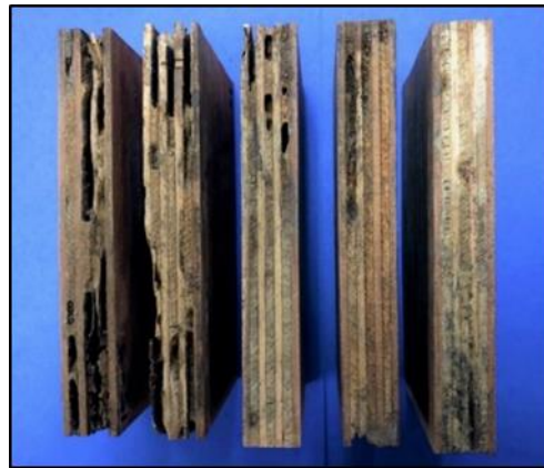
Fig. 12. The 3-mm hoop crossbands were badly damaged in some instances
