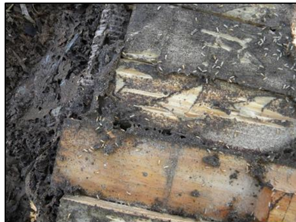
Fig. 3. Timber placed atop the aggregation trench was heavily infested with C. acinaciformis
