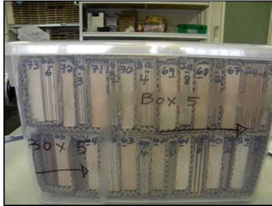
Fig. 2. Plywood test blocks and pine feeder sapwood blocks positioned in an exposure box
