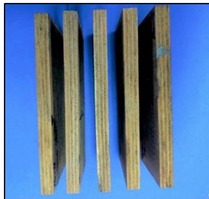
Fig. 11. Test blocks with a CYP longband and a 1.0-mm hoop pine crossband were undamaged
