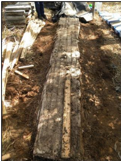
Fig. 3. Timber placed atop the aggregation trench was heavily infested with C. acinaciformis
