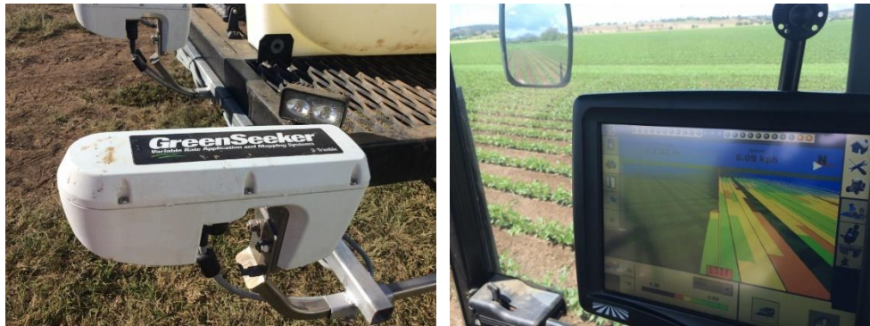
Figure 4. Greenseeker operation. A) tractor-mounted GreenSeeker® and B) real time display of crop sensing data. Source: Limpus, et al. (2016)
