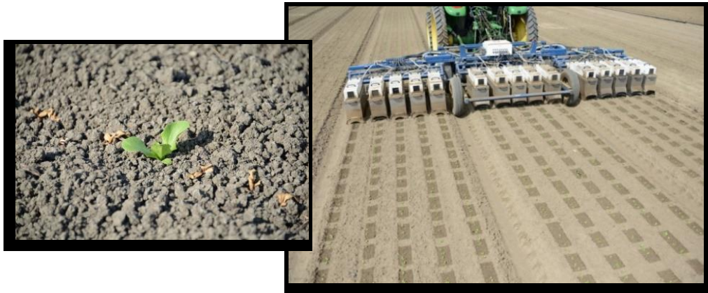
Figure 34. LettuceBot for precision lettuce thinning. Note the selection of the green leaves and the targeted-sprayed unwanted leaves (brown leaves). Source: (Blue River Technology)
