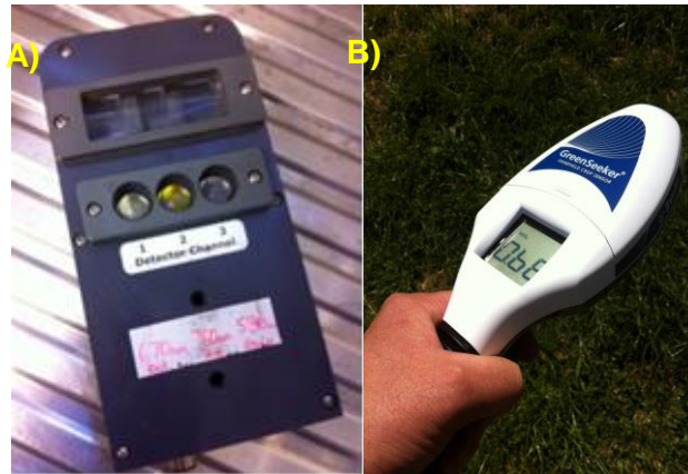
Figure 2. Examples of proximal and active systems 6 . A) CropCircle™ ACS-470; B) GreenSeeker Hand held (GSHH).
