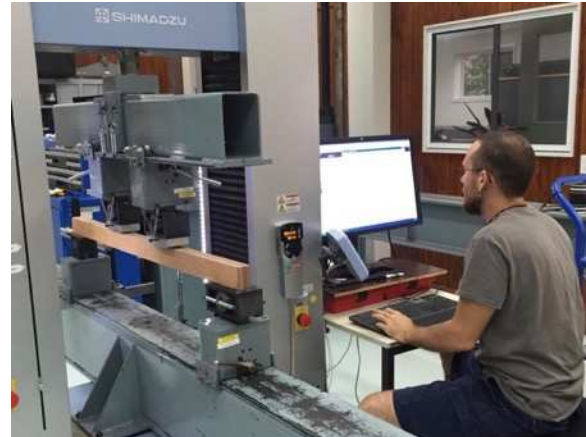
Figure 33: Testing LVL sections
