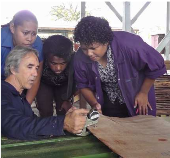
Figure 8: Accessing veneer thickness during Trial 3.
