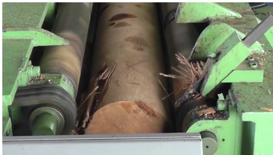
Figure 4: A senile coconut log in a spindle-less lathe
