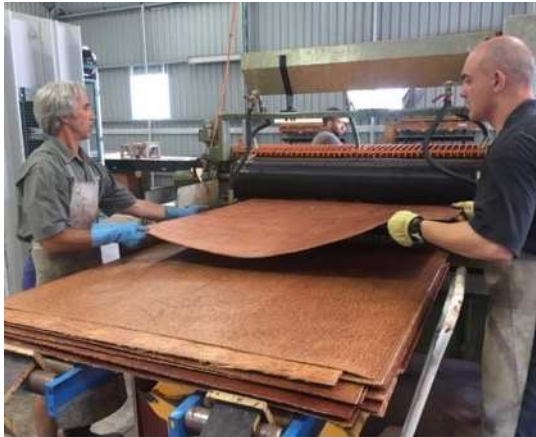
Figure 32: Applying glue to coconut veneer sheets
