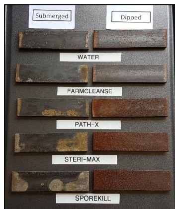
Figure 6: Unpainted steel, submerged in solution (left), dipped frequently (right)
