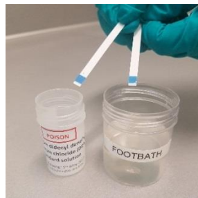
Figure 1: Test strips dipped into 1% standard solution and footbath sample simultaneously
