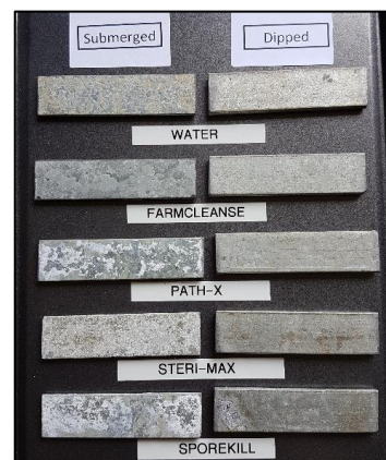
Figure 10: Galvanised steel, submerged in solution (left), dipped frequently (right)
