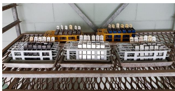
Figure 4: Metals placed on racks and exposed to field conditions
