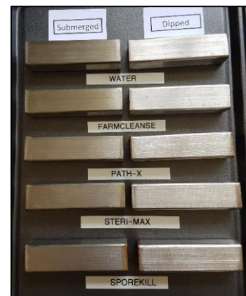
Figure 8: Stainless steel, submerged in solution (left), dipped frequently (right)
