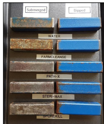
Figure 7: Painted steel, submerged in solution (left), dipped frequently (right)
