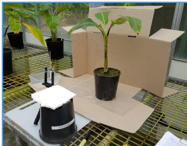
Figure 1.1: Potted Dwarf Ducasse plants were placed in front of a plain cardboard background and 30 cm from the camera (not pictured) as the standard set-up for taking NDVI pictures of the pseudostem. A piece of polystyrene was placed behind for the thermal photos.
