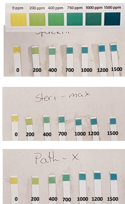
Figure 1: Calibration of Precision Laboratories High Level QAC test strips
