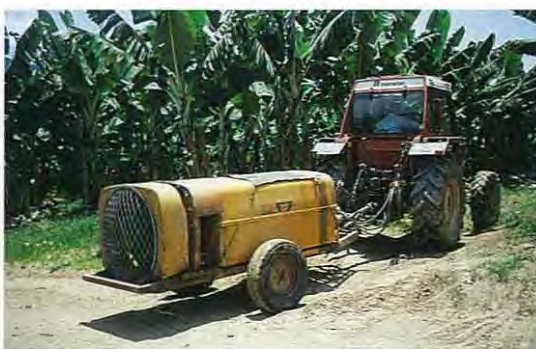
Figure 7.3: Large air-blast sprayer suitable for larger plantations
