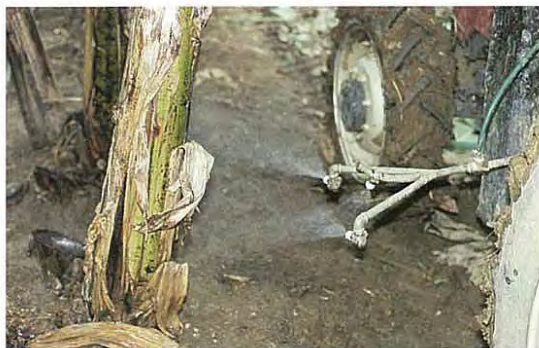
Figure 7.5: A simple spray unit for band application
