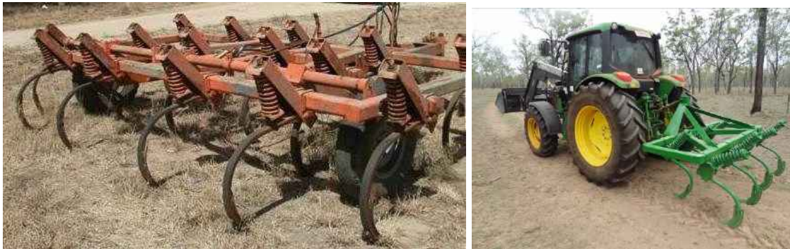
Figure 9. Chisel ploughs: L. Trailed hydraulic type; and R. A 3-point linkage mounted type.
