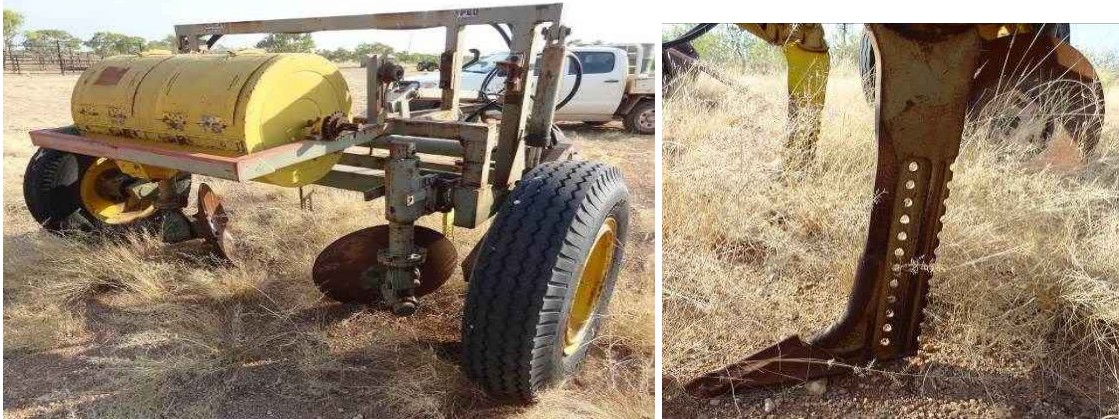
Figure 13. Twin off-set discs with deep ripping tynes and roller seeder for shallow ponding bank regeneration of scalds (machines used in the Ord and Fitzroy River regeneration programs in WA).
