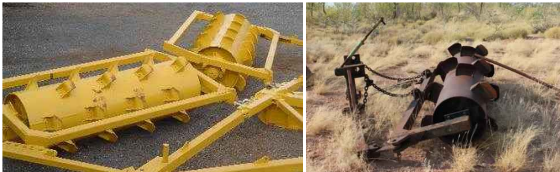
Figure 10. L. Crocodile plough seeder ex. hoopersengineering.com ; R. Single cylinder crocodile plough seeder (Fitzroy River WA regeneration)
