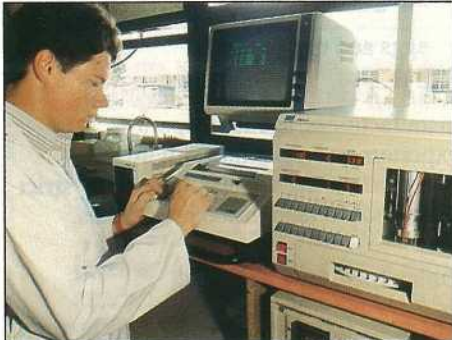
Plate 3. Analysis of sugars in food by high performance liquid chromatography.
