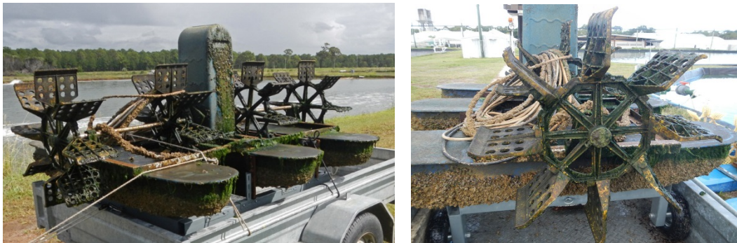
Figure 7. Chenta 2hp paddlewheel tested. Heavily fouled with barnacles and algae. Dense covering of barnacles on the float submersed surfaces, algae (filamentous and slime) and barnacles on the paddles and upper surfaces. Paddles not heavily fouled, with little filamentous algae but covered in dark biofilm. Total weight of fouling in air = 35.1kg.
