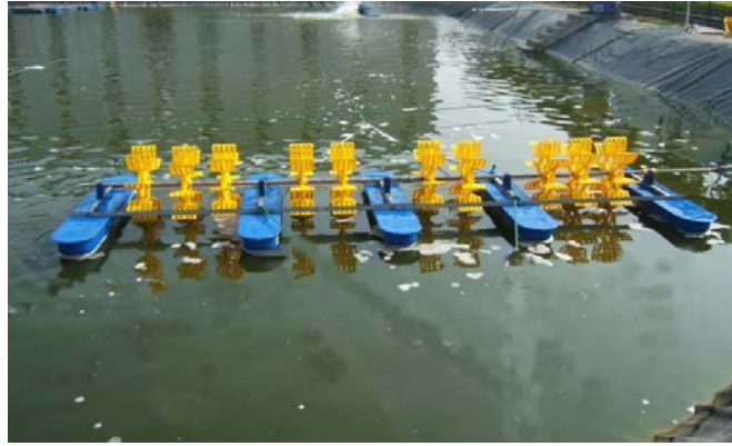
Figure 8. Long arm paddlewheel driven from the bank.
