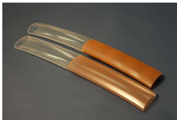
Figure 3. Copper coating on polyurethane at two densities. Photo from (King, et al. 2010).
