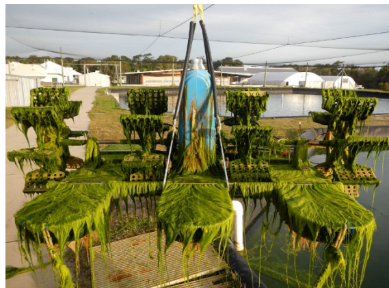
Figure 6. Futi 2hp paddlewheel tested. Heavily fouled, predominantly filamentous algae ( Ulva sp). Total wet weight of fouling in air = 20.7kg. As algae covers the upper surfaces this weight will be a large underestimate of additional weight loading during operation due to entrapment of water.
