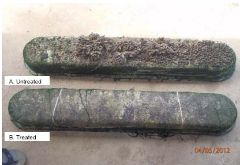
Figure 5. Floats from a paddlewheel that was installed in a prawn pond in Thailand. Weight of mussels on untreated float was approximately 10kg. Photo from Charlton 2012.
