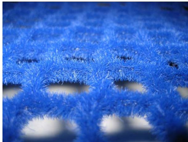
Figure 7. Thorn-D physical biofouling deterrent as applied to fish cage netting (Micanti 2012).
