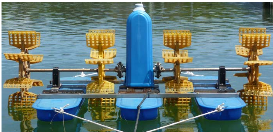
Figure 10. Front profile of a standard Taiwanese style paddlewheel showing numerous corners and curves and profiles on larger surfaces. Photo D. Mann.
