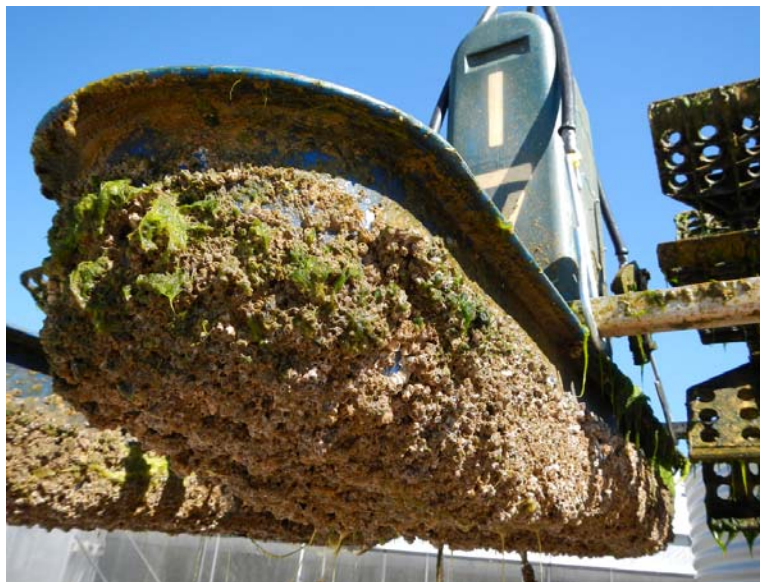
Figure 2. Algal fouling on upper surfaces and submersed surfaces of prawn farm paddlewheels. Photos D. Mann.
