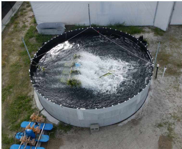
Figure 1. Oxygenation test tank. Under test conditions the tank contained 40,000L of fresh water at 1.21m deep. Paddlewheels took up to 2h to return water DO to near saturation from the deoxygenated state.
