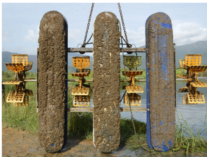
Figure 15. Typical barnacle cover after 3 months operation, observed in the trial on each of the three float surface treatments. From left- uncoated, AFwax, Protecta-hull.
