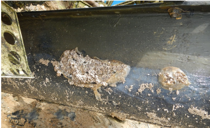
Figure 16. Barnacle growth in patches of ruptured Protecta-hull coating. Note that the barnacles are able to grow partially covered by the delaminated coating.
