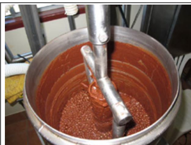
Figure 42. Programmable chocolate maker (ball grinder) with heated water jacket. A view of stainless balls used to reduce particle size
