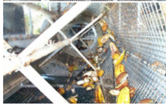
Figure 16. Pod and bean separator tumbler
