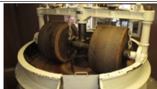
Figure 36. The restored melanger (granite rollers) used for grinding cocoa nibs and sugar for large scale (250 kg) chocolate batches
