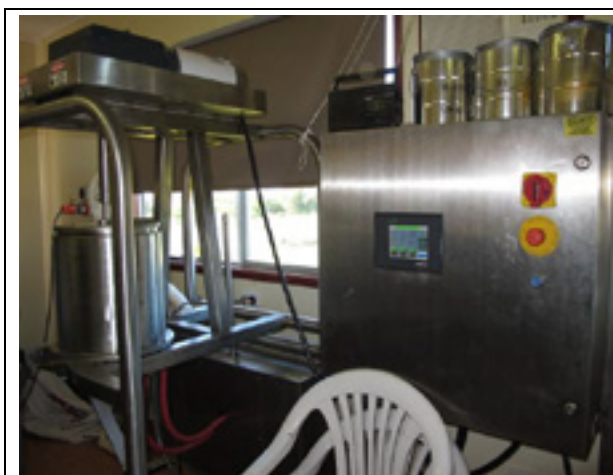
Figure 42. Programmable chocolate maker (ball grinder) with heated water jacket. A view of stainless balls used to reduce particle size
