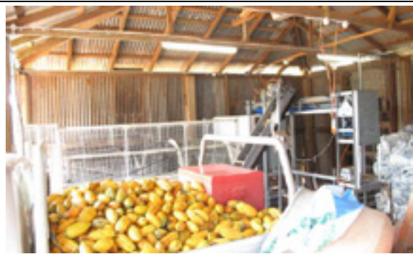
Figure 13. Load of cocoa pods ready for processing with the cocoa pod splitter and bean separating unit in the background
