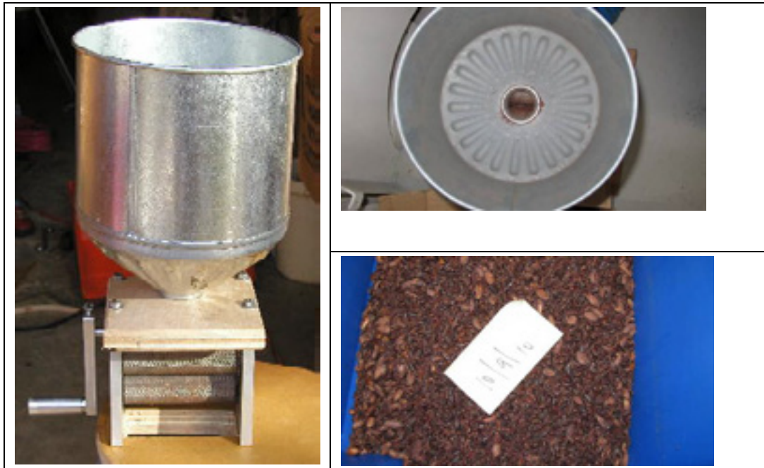
Figure 34. Crankandstein mill side on and top view and Crushed beans from a north Queensland batch ready for winnowing
