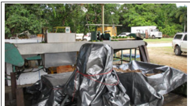
Figure 26. Fermentation vessel's covered in a tarpaulin to aid with heat retention
