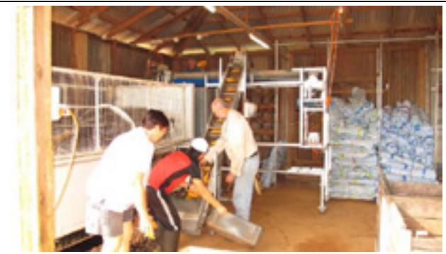
Figure 14. Feeding pods onto the pod splitter via a pod elevator
