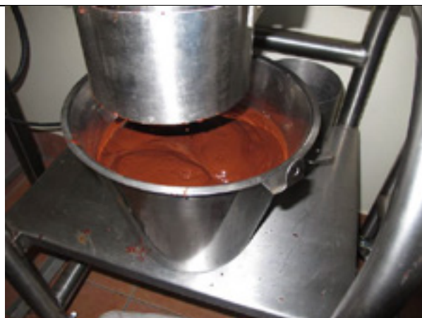
Figure 41. Nib grinder and the consistency of the cocoa mass (liquor) after it has passed through the final sieve
