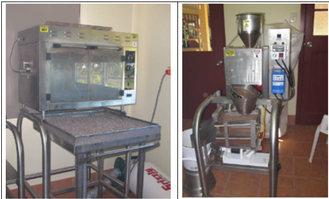
Figure 40. Bean roasting unit with a drum roller (behind glass doors) and bean cooling tray (left) and a 15 kg/hr bean cracking and winnowing unit (right)
