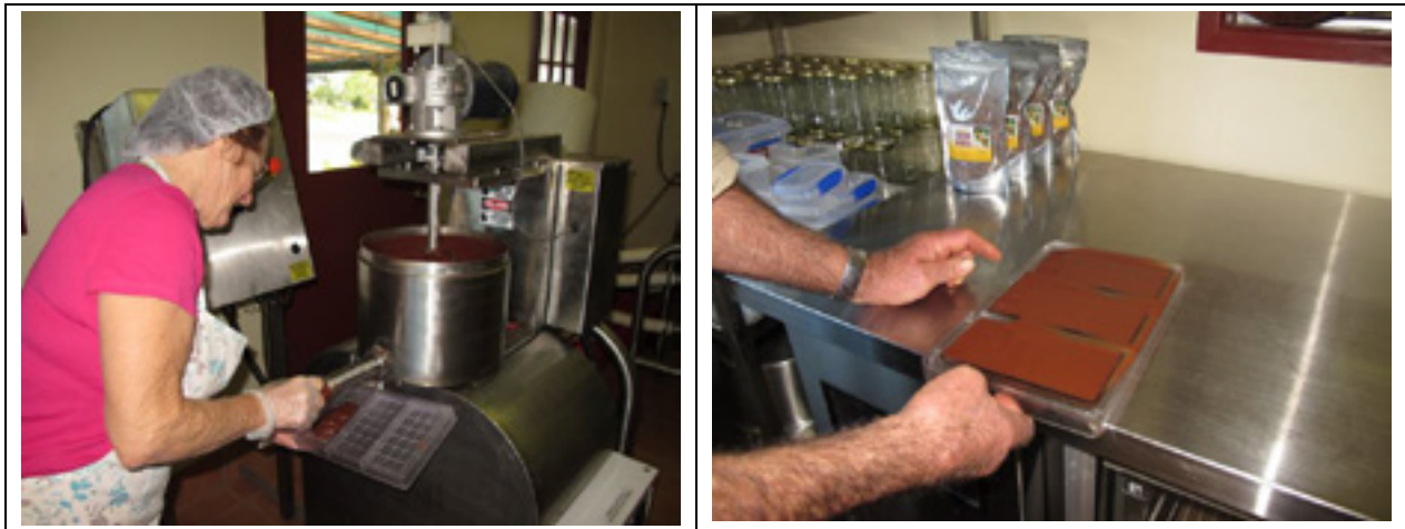
Figure 43. Pouring chocolate into the mould from the tempering machine (left) and removing trapped air in the moulds prior to cooling
