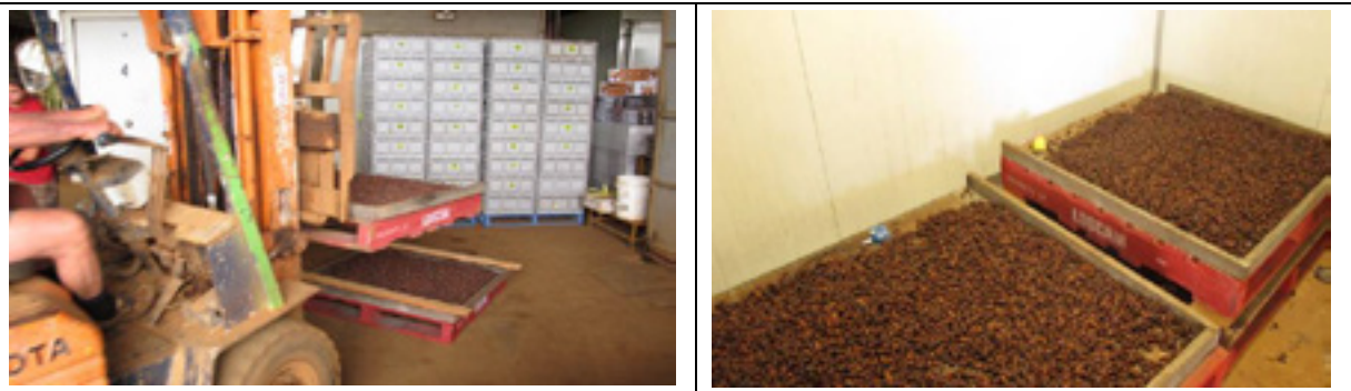
Figure 20. Bean drying on palletised drying trays occurring in the new high temperature humidity controlled rooms
