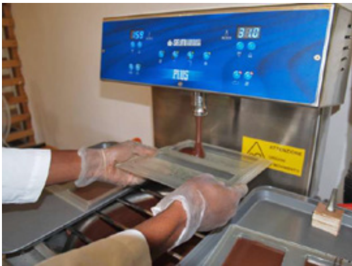
Figure 39. Selmi Plus mechanical tempering devise used for larger batch sizes
