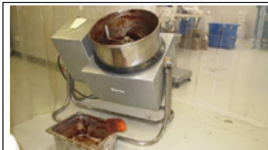
Figure 35. The Santha granite roll mill used for grinding cocoa nibs and sugar for small volumes of beans (1-2 kg) chocolate batches
