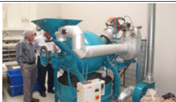
Figure 32. Barth Sirocco ball roaster (restored)
