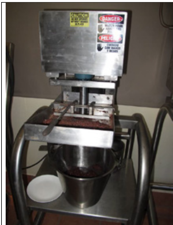
Figure 41. Nib grinder and the consistency of the cocoa mass (liquor) after it has passed through the final sieve
