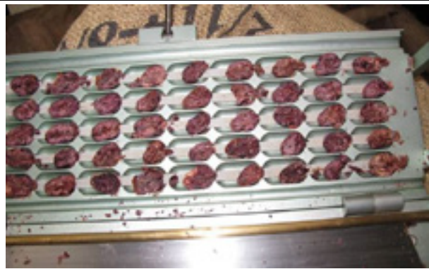
Figure 30. A Magra “Cut Test” guillotine
