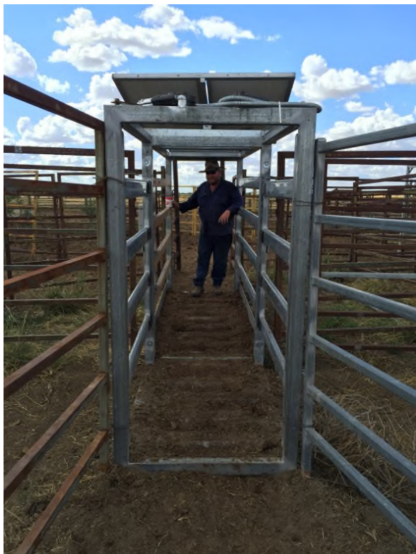
Figure 3. Large amounts of dirt collecting on the floor of the WOW unit raises concerns about the accuracy of the weight data collected and will continue to be closely monitored.
