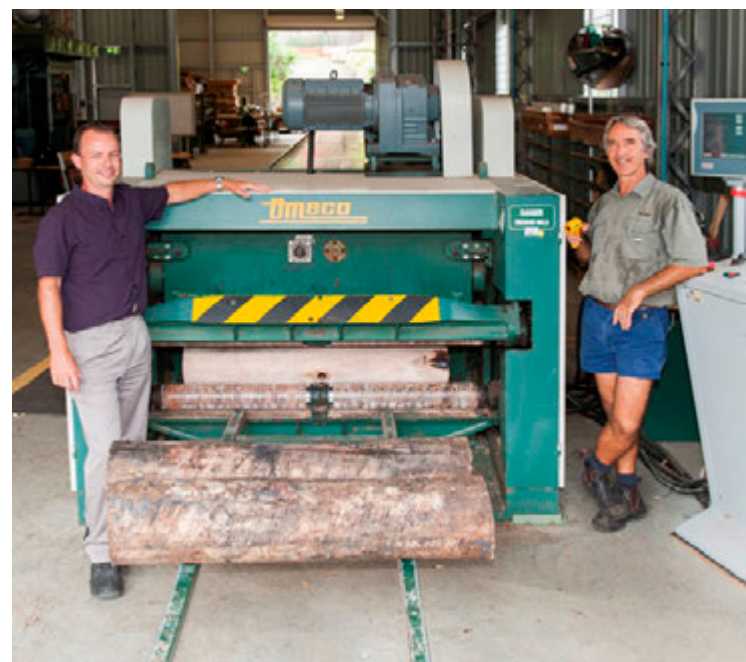
Research staff with a spindleless lathe at the Salisbury Research Facility
