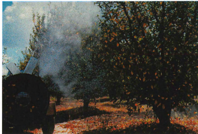
Figure 12. An airblast machine spraying apple trees. The sprayer is fitted with top baffles so the air is parted and directed to match the tree height. This attachment reduces spray loss between rows.
