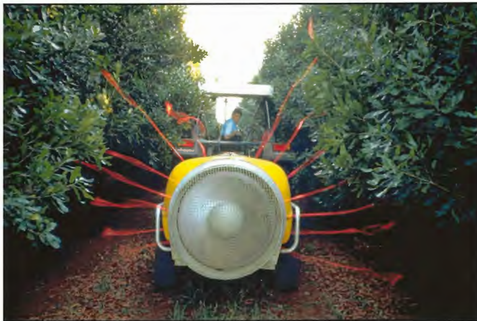
Figure 1. A low profile airblast sprayer shown in a macadamia orchard with no hedging or tree shaping. The ribbons show the most likely path of droplets from the various nozzle positions. Much of the spray will be intercepted by foliage in the lower part of the tree.
