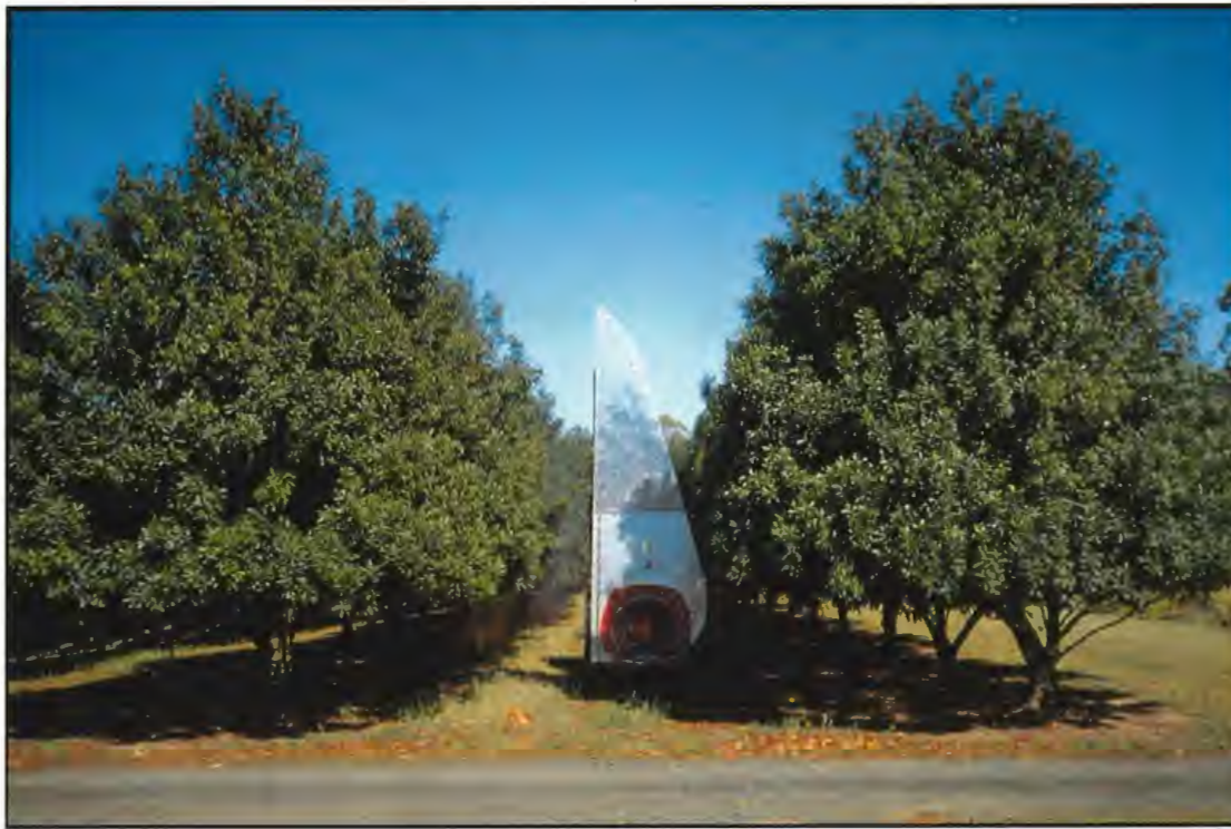
Figure 6. Examples of airblast tower sprayers (a) Cropland's Tri-fan, a two sided tower with 3 fans, (b) Jan-ell's Jen-Tech-Raider 2000, a two sided with two separate fans and (c) the Hardi eco-tower, a single sided tower.
