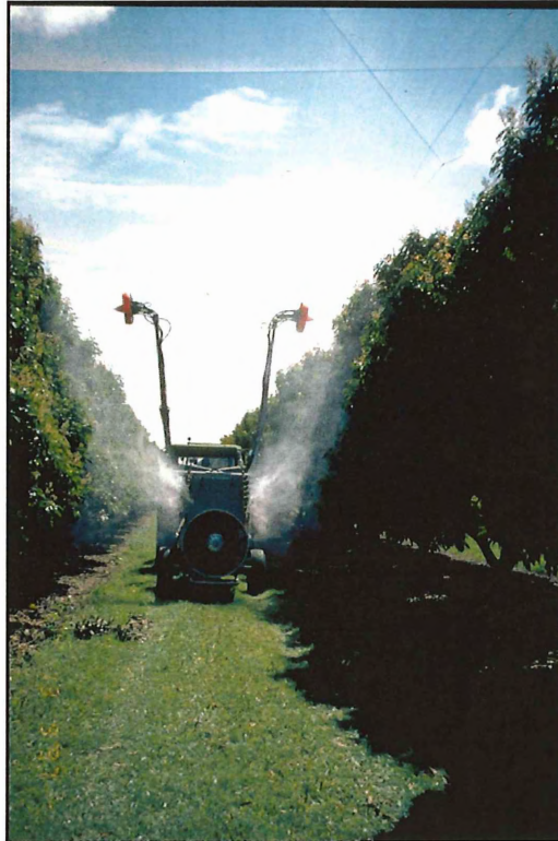
Figure 10. A combination of two sided airblast with two Hydra fan heads mounted on extended arms.
