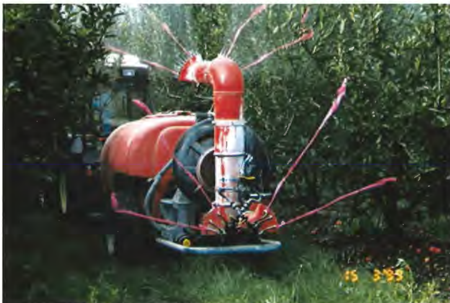
Figure 7. A custom built, low profile airblast sprayer, comprising of two axial fans. The unit is not powered by the tractor but a separate diesel motor that operates the two fans and pump unit.
