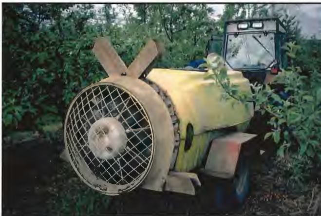
Figure 3. Some examples of different low profile airblast sprayers used by many orchard industries. Air baffles have been fitted in sprayers a,b and d to manipulate the air flow direction from the top of the sprayer manifold.
