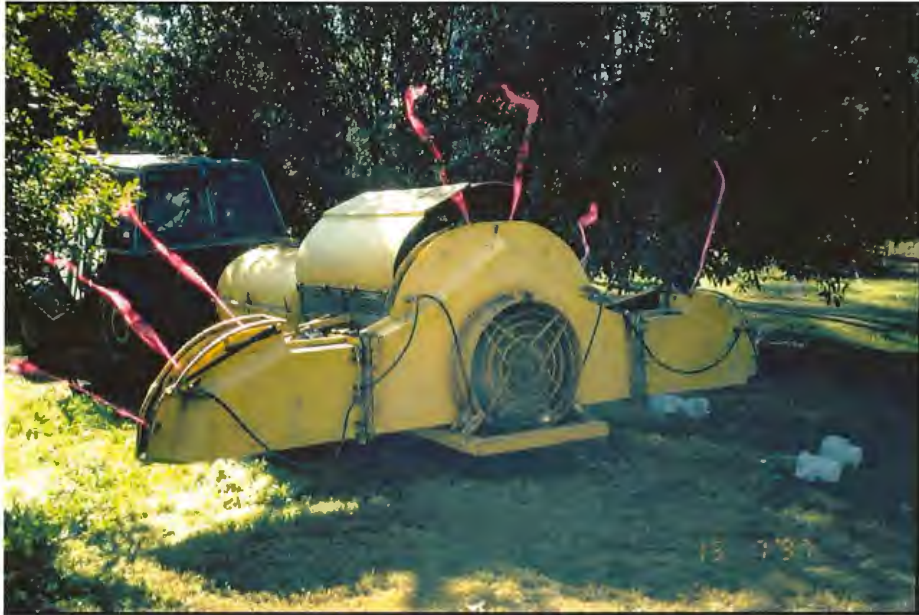
Figure 7. A custom built, low profile airblast sprayer, comprising of two axial fans. The unit is not powered by the tractor but a separate diesel motor that operates the two fans and pump unit.
