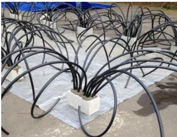
A simple 'Jack' constructed from pipe and PVC tube and a more complex design after some time in the water. The benefit of the Jack is that it will always create vertical structure when deployed due to its design.
