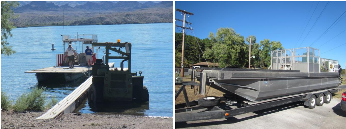
Some of the specialist equipment used to deploy habitat structures: the flat-deck habitat barge and tractor at Lake Havasu, and the tilt-deck habitat barge at Table Rock Lake.
