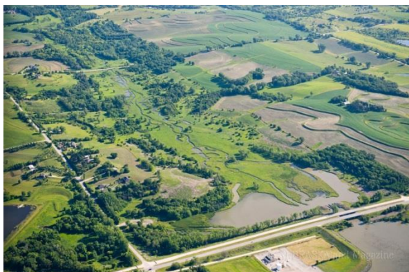
Constructed wetlands designed to trap sediment, improve water quality and create habitat and nursery areas for fish (images NGP)
