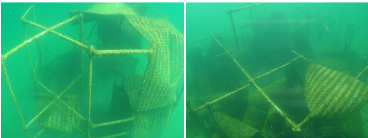
Snow fencing detaching from the PVC pipe frame
