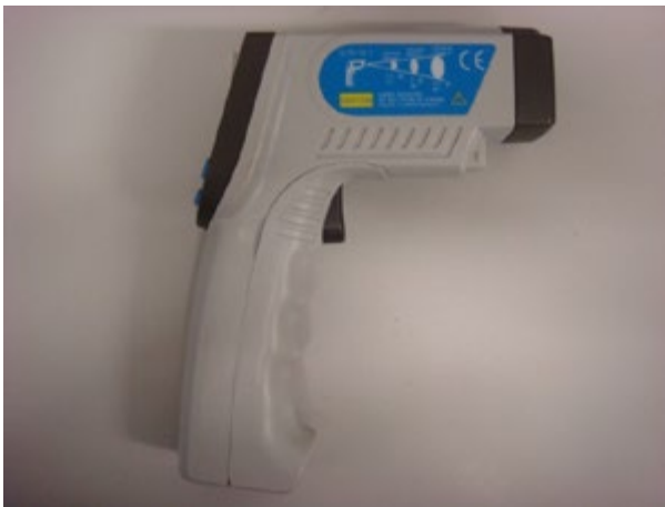
Figure 9 An example of an infrared laser thermometer that can be used to measure the surface temperature of fan belts, sheaves, bearings or motors to measure if they are running hot
