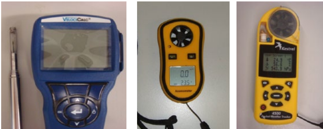
Figure 4 Different types of anemometer that are available: left—Hot-wire anemometer; middle and right—vane anemometers
