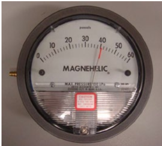
Figure 1 Dwyer Instruments Magnehelic® differential pressure gauge
