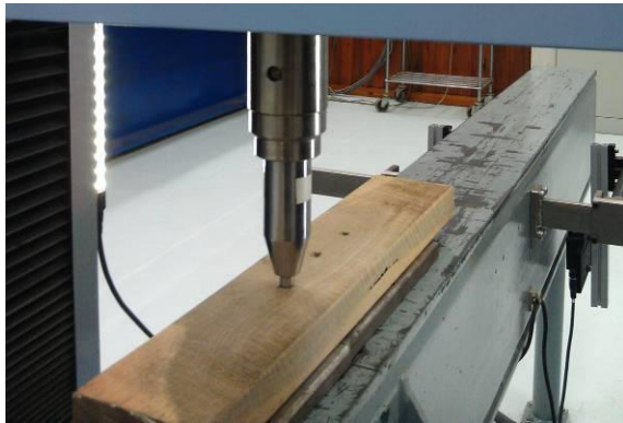
Image 15: Hardness testing on a board sample (force measured at three points per sample on the tangential surface).
