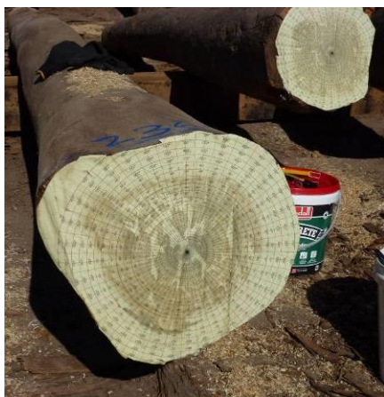
Image 8: Template glued on large log-end allowing board position within a log to be quantified.
