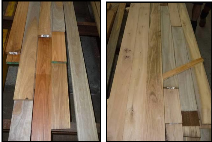
Image 17: Example of visual appearance for Parkside production native timber (left) and plantation timber (right)
