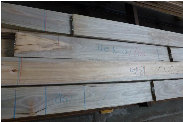
Image 13: Visually grading timber.
