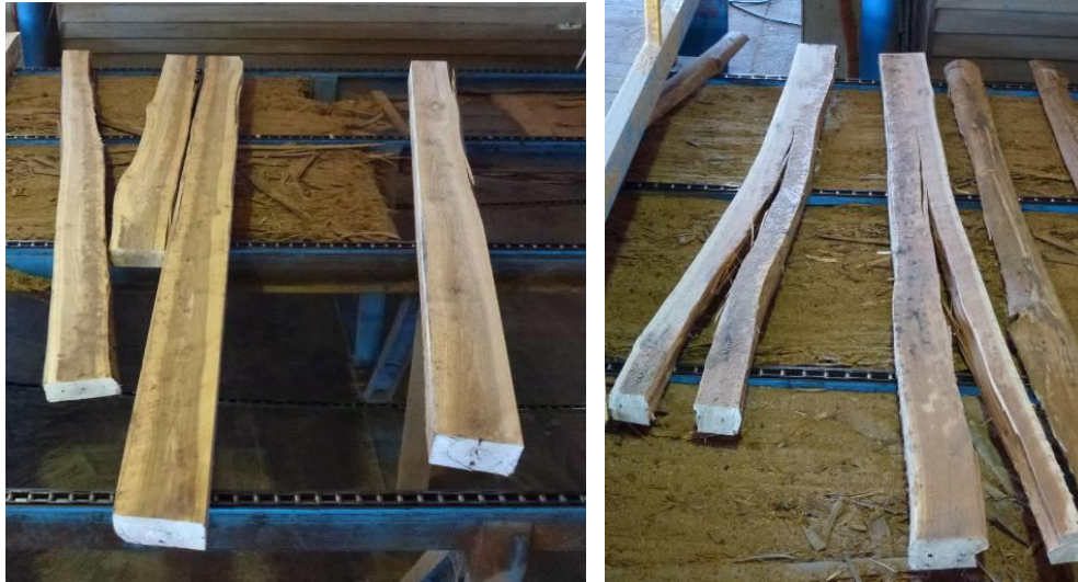
Image 16: Examples of cant after primary break-down: left) CCV did not exhibit problems with splitting; right) log-end splitting in GMS, the consequence of sawing was a cant that was too thin relative to the log diameter.
