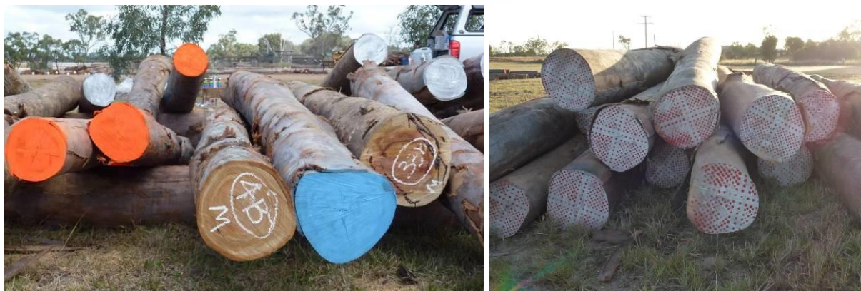
Image 9: Colour coding of logs and separating into batches. Paint applied on small ends, poker dots used to distinguish top logs (right).
