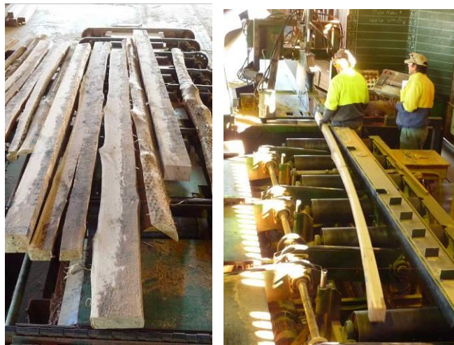
Image 11: Processing thicker flitch wane and cant (left) through the Gibson re-saw bench (right). Note the timber bowing distortion in the cant, which was not rotated during sawing.
