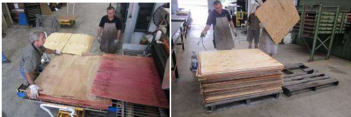
Image 10: Applying adhesive to the veneer (left) and water spraying plywood panels after manufacture (right)
