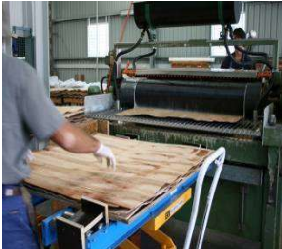
Image 8: Veneer cross bands having adhesive applied (left) and panels being cold pressed (right)
