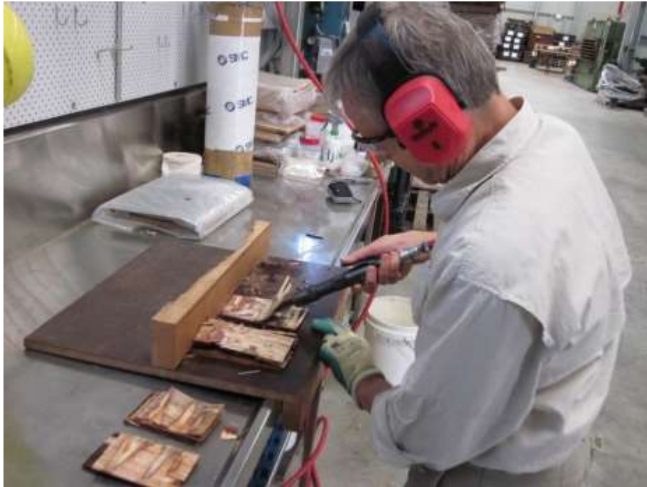
Image 4: Pneumatic chisel used to separate veneers
