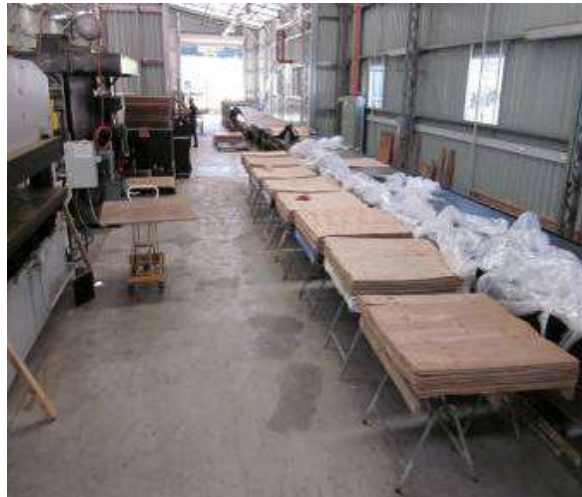
Image 7: Reference veneer including acoustic grade (left) and veneer prepared for sequential assembly (right)
