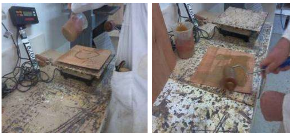
Image 1: Accurately measured adhesive added to veneer (left) before being spread using a hand roll applicator (right)
