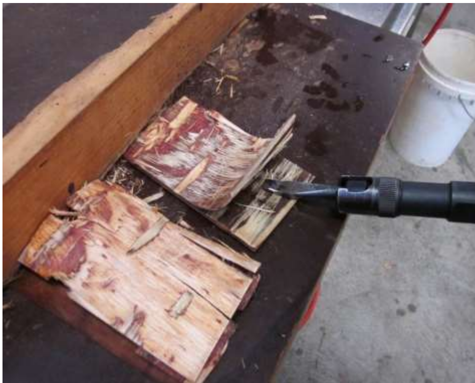
Image 5: Separated veneers facilitate assessment of wood fibre failure
