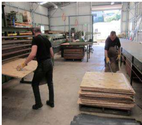
Image 9: Hot pressing panels (left) and water spraying plywood panels after manufacture (right)
