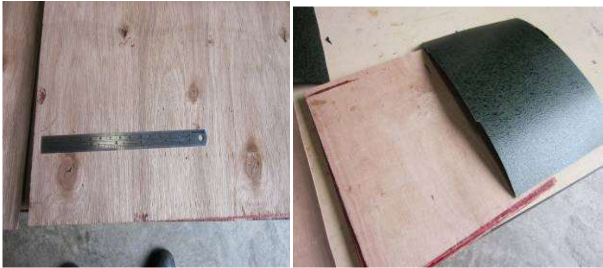
Image 3: Knotty faced B grade face veneer (left) and A grade clear faced veneer (right)
