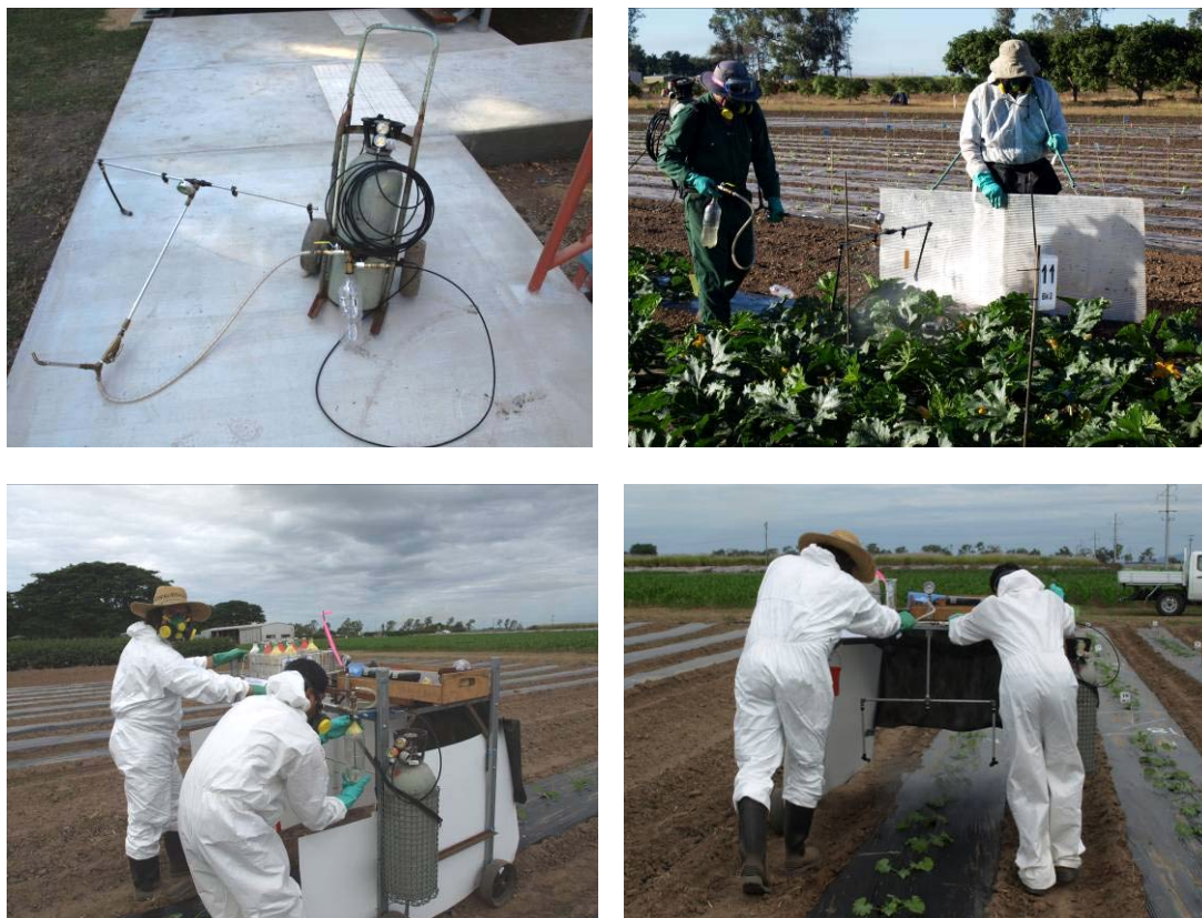
Figure 22. Trolley and backpack CO 2 -pressurized sprayers used in 2009 (top left and right) and unit mounted on wheels (bottom left and right) used in 2010. The spray products were prepared in 1-L plastic bottles, which were attached to the header of sprayer before treating the 10-m 2 plots.
