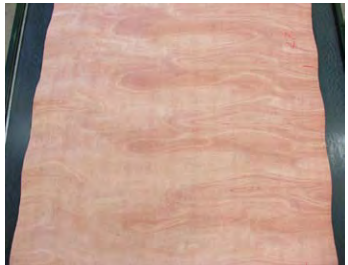
Figure 7. Veneer from a log harvested at 20 years of age from a stand at Burdekin Agricultural College, Queensland. The colour darkens on exposure. K. Harding
