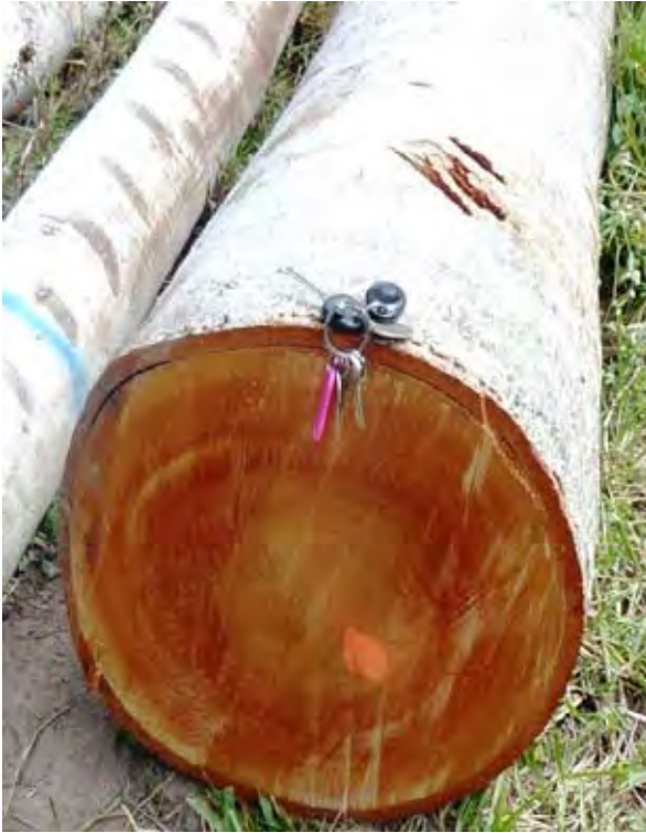
Figure 8. Logs from thinning of a 10-year-old, farm forestry stand in coastal lowlands north of Townsville, Queensland. Note the high proportion of dark-coloured wood of the log end. K. Harding.
