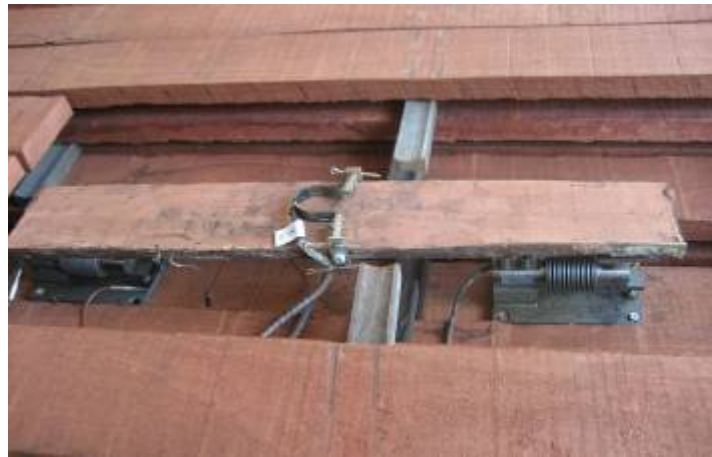
Plate 5. Position of flying wood test board during drying
