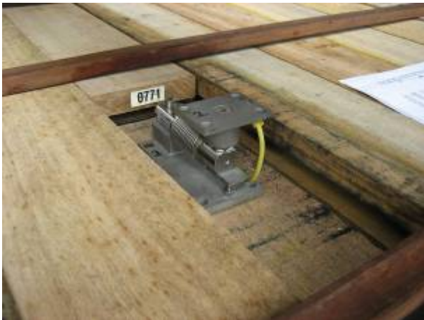
Plate 8. Load cell placement
