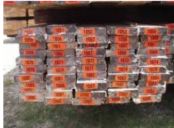
Plate 2. End coated and labelled boards
