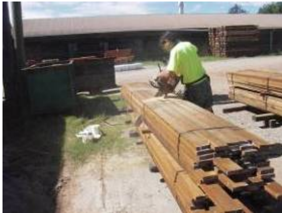
Plate 1. Preparation of end matched boards
