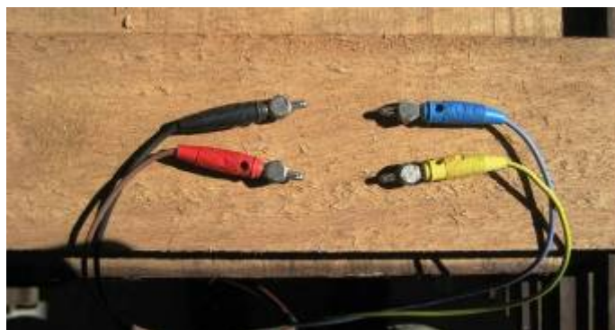
Plate 3. MC resistance probes inserted into a test board
