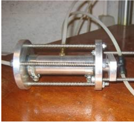
Figure 7. ALU-CHA system for longitudinal samples
