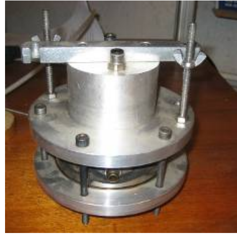
Figure 8. ALU-CHA system for transverse samples
