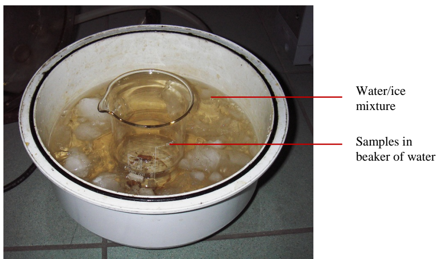
Plate 15. Samples prepared for vacuum saturation (container uncovered for photo)
