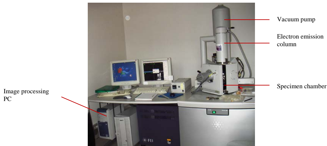
Plate 12. FEI Quanta 200 3D environmental electron scanning microscope.
