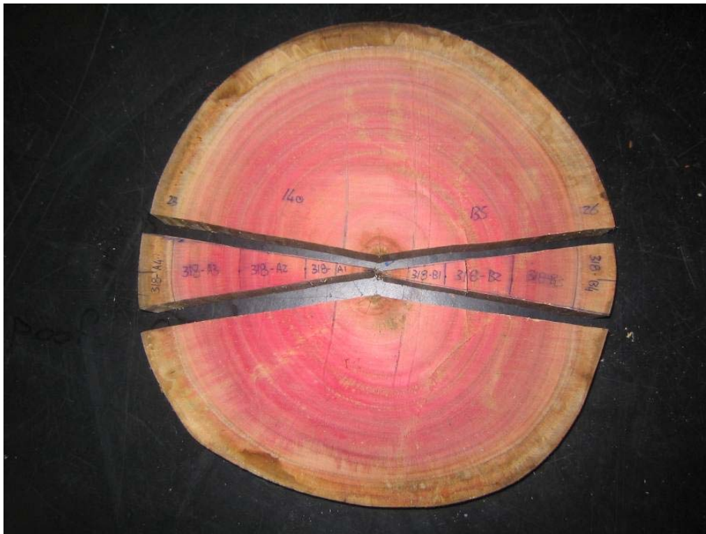
Plate 3. Example of disc with coloured staining showing heartwood (pink) and sapwood boundary 3 .
