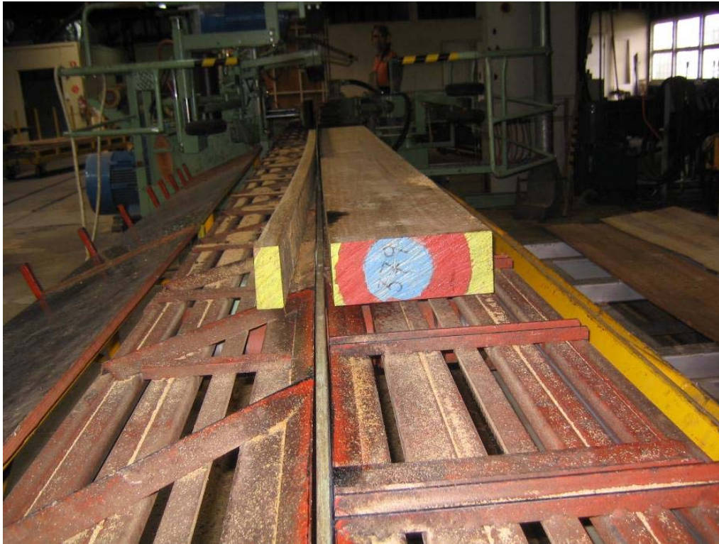
Plate 2. Processing the centre cant to remove target boards.
