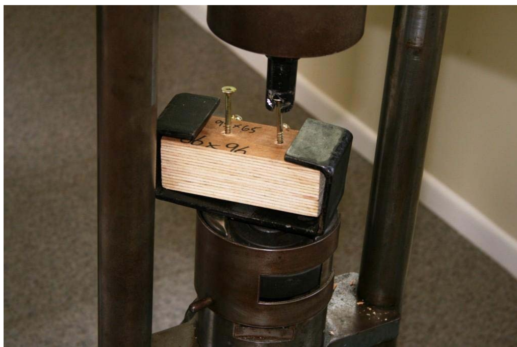
Plate 5. Universal test machine set up for the nail and screw withdrawal test.
