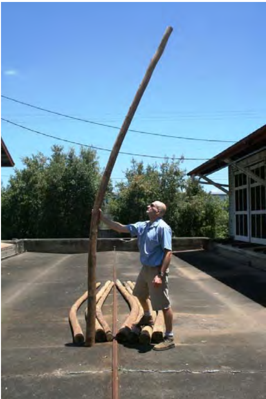
Plate 7. Retained curvature 7 days after release from the bending form.
