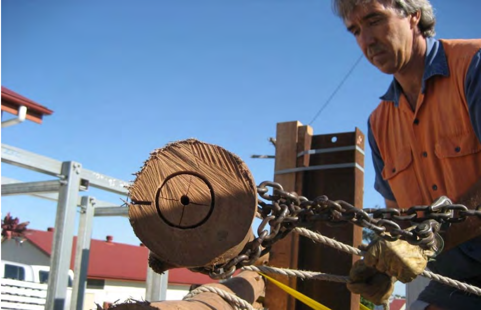
Plate 6. Steamed logs fixed onto the bending form. Note the ring groove and external kerf treatment used to limit end splitting.
